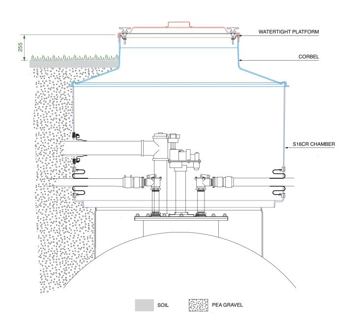
1.5m diameter sump with collar ring, corbel, stainless steel retainer ring and watertight platform. For green area application.
