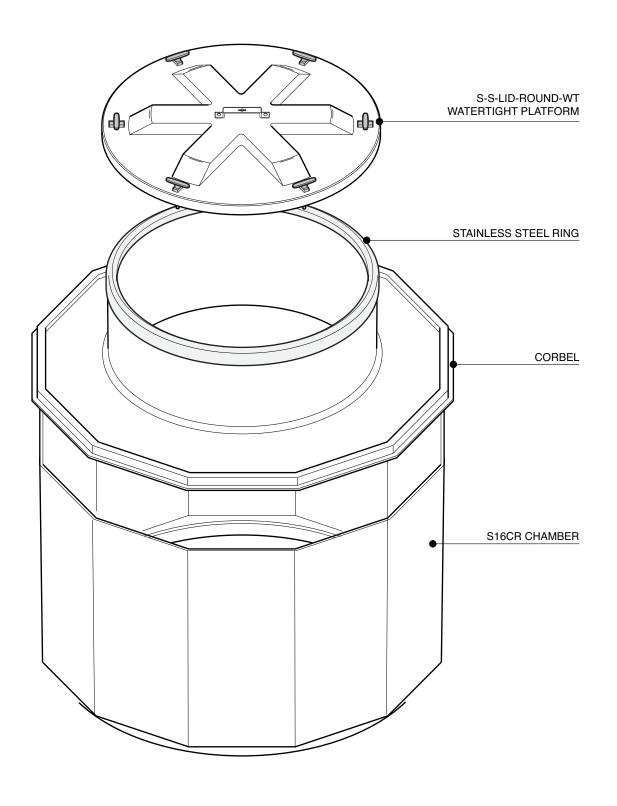
1.5m diameter sump with collar ring, corbel, stainless steel retainer ring and watertight platform. For green area application.
