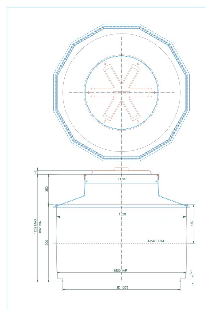
1.5m diameter sump with collar ring, corbel, stainless steel retainer ring and watertight platform.
