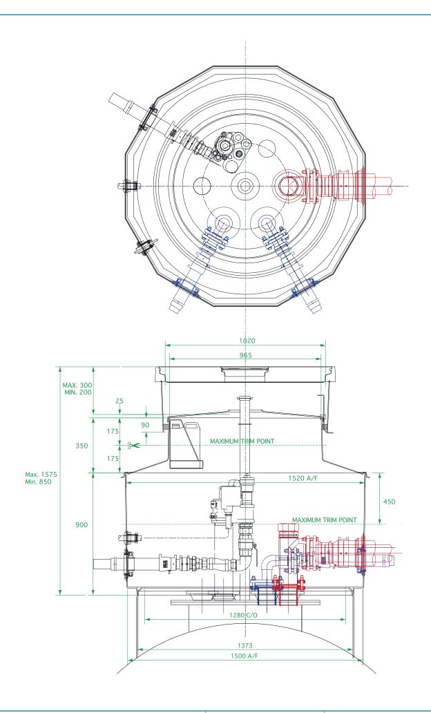
1.5m dia twelve sided sump with collar ring base. corbel, skirt, non structural internal lid with dipstick hole. 1020mm dia flat sealed cover with central sealed cover and frame.
