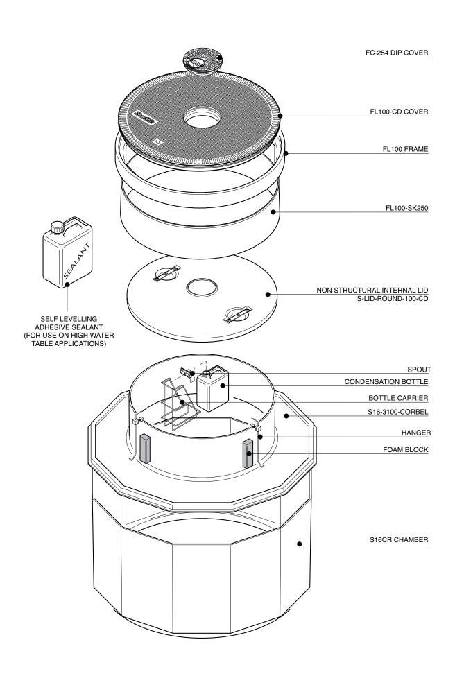
1.5m dia twelve sided sump with collar ring base. corbel, skirt, non structural internal lid with dipstick hole. 1020mm dia flat sealed cover with central sealed cover and frame.
