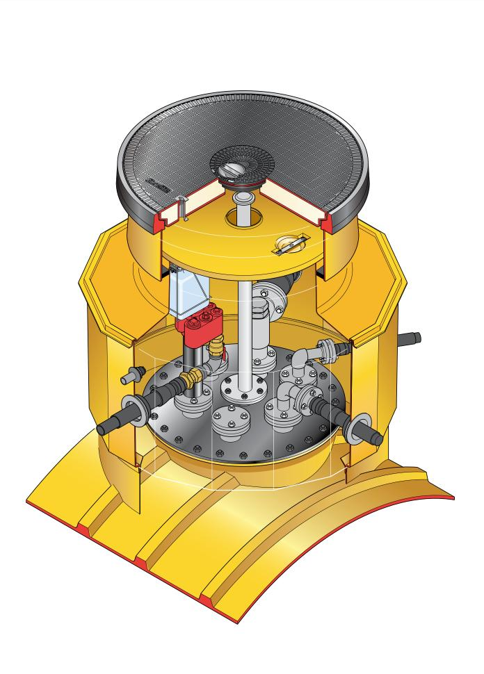
1.5m dia twelve sided sump with collar ring base. corbel, skirt, non structural internal lid with dipstick hole. 1020mm dia flat sealed cover with central sealed cover and frame.
