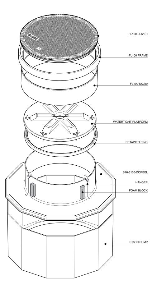
1.5m diameter 12 sided sump with collar ring base, corbel, adjustable height skirt, internal watertight platform, round 1020mm flat sealed cover and frame.
