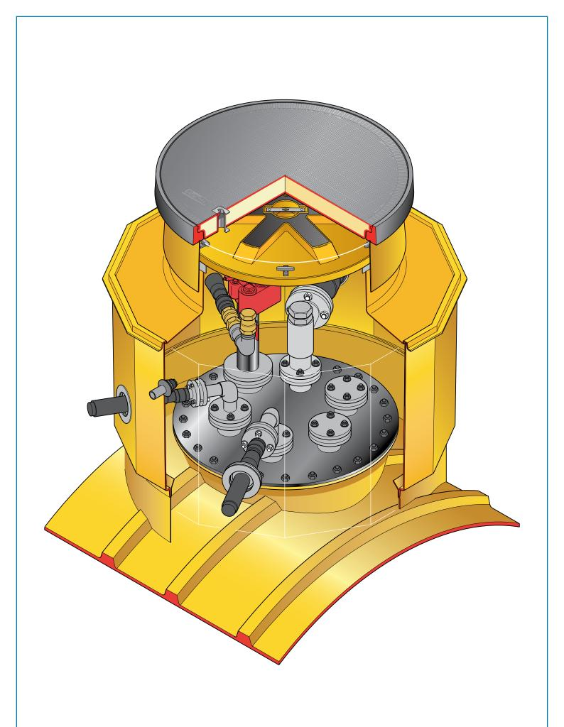
1.5m diameter 12 sided sump with collar ring base, corbel, adjustable height skirt, internal watertight platform, round 1020mm flat sealed cover and frame.
