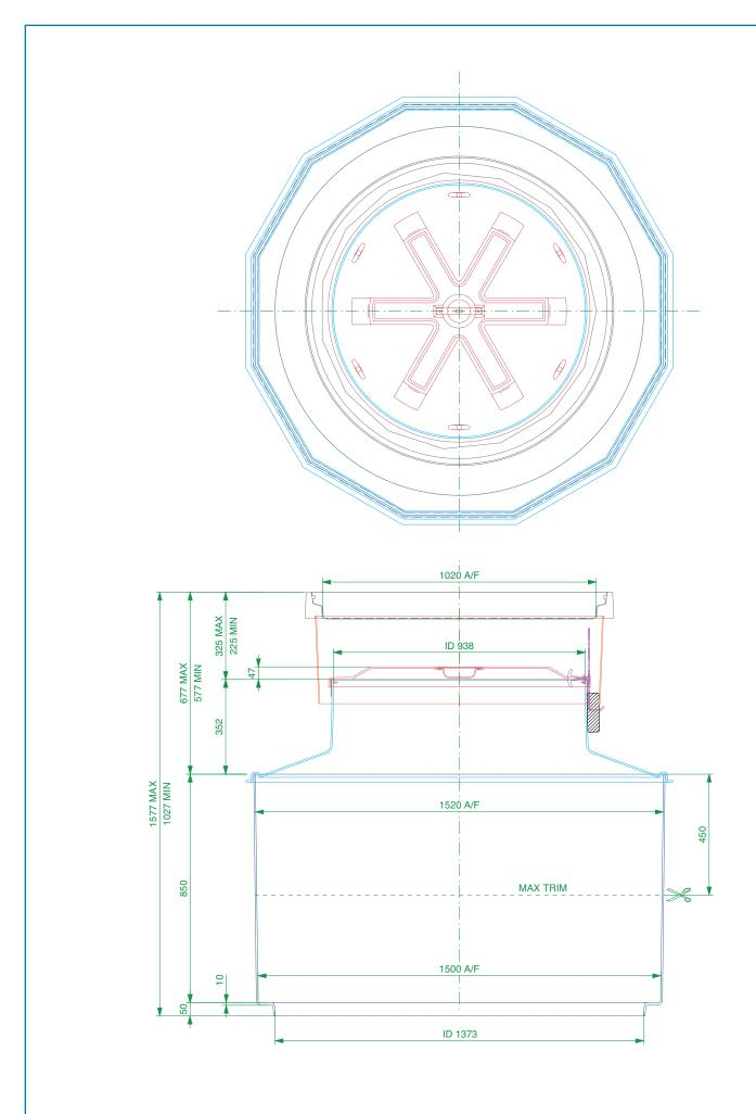
1.5m diameter 12 sided sump with collar ring base, corbel, adjustable height skirt, internal watertight platform, round 1020mm flat sealed cover and frame.
