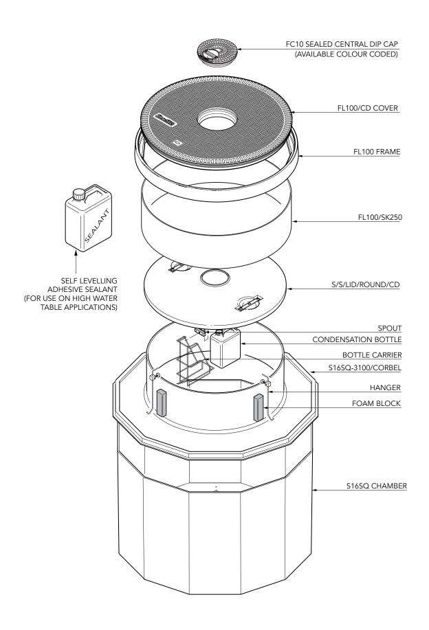
1.5m diameter 12 sided sump with solid base and manway lid adaptor, corbel, adjustable height skirt, internal lid, and round 1020mm flat sealed cover with central dip cover and frame.
