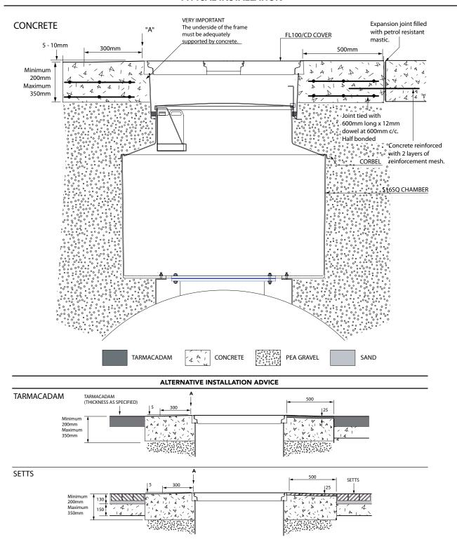
1.5m diameter 12 sided sump with solid base and manway lid adaptor, corbel, adjustable height skirt, internal lid, and round 1020mm flat sealed cover with central dip cover and frame.
