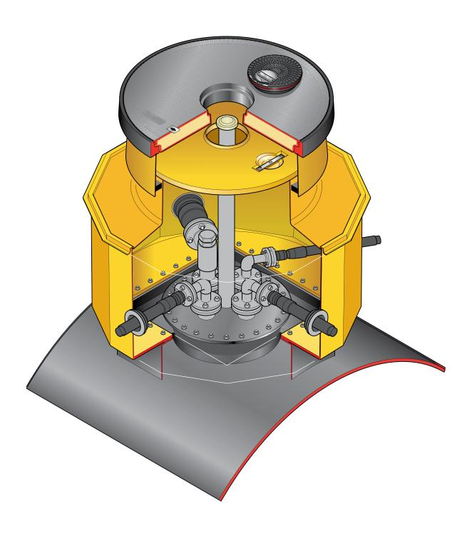
1.5m diameter 12 sided sump with solid base and manway lid adaptor, corbel, adjustable height skirt, internal lid, and round 1020mm flat sealed cover with central dip cover and frame.
