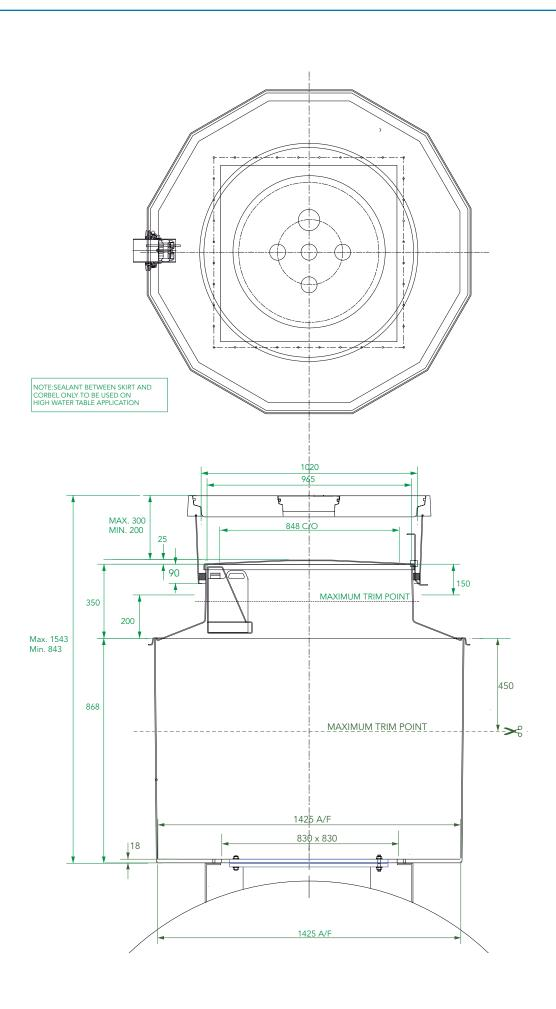
1.5m diameter 12 sided sump with solid base and manway lid adaptor, corbel, adjustable height skirt, internal lid, and round 1020mm flat sealed cover with central dip cover and frame.
