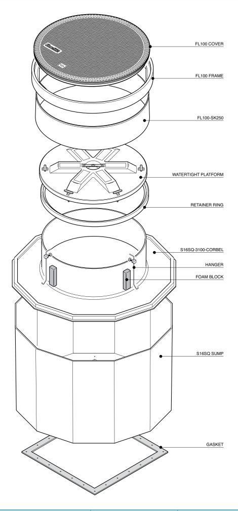
1.5m diameter 12 sided sump with a square flange, corbel, adjustable height skirt, internal watertight platform, round 1020mm flat sealed cover and frame.
