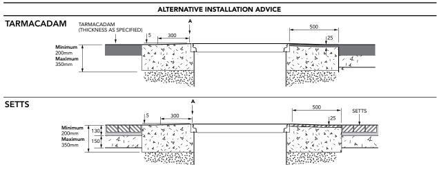
1.5m diameter 12 sided sump with a square flange, corbel, adjustable height skirt, internal watertight platform, round 1020mm flat sealed cover and frame.
