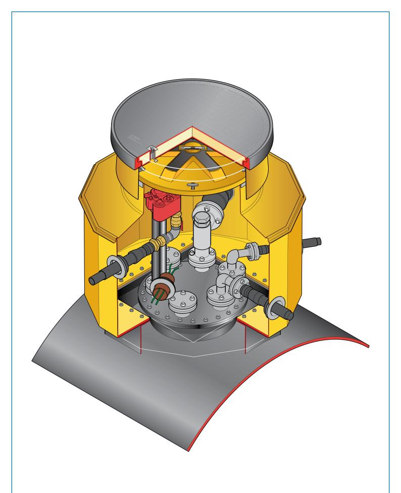
1.5m diameter 12 sided sump with a square flange, corbel, adjustable height skirt, internal watertight platform, round 1020mm flat sealed cover and frame.
