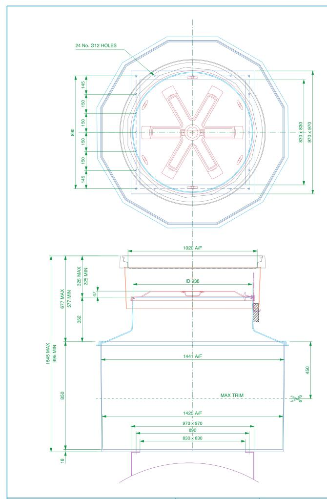
1.5m diameter 12 sided sump with a square flange, corbel, adjustable height skirt, internal watertight platform, round 1020mm flat sealed cover and frame.
