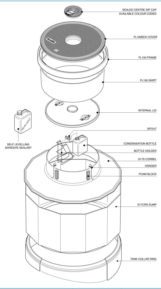
1.7m diameter stackable sump with collar ring base, stackable corbel, non-structural internal lid, adjustable height skirt, round 1020mm flat sealed cover and frame.
