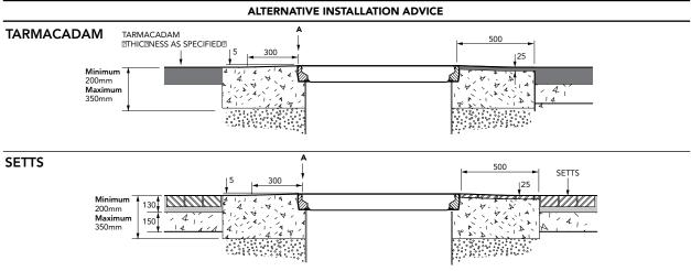
1.7m diameter stackable sump with collar ring base, stackable corbel, non-structural internal lid, adjustable height skirt, round 1020mm flat sealed cover and frame.
