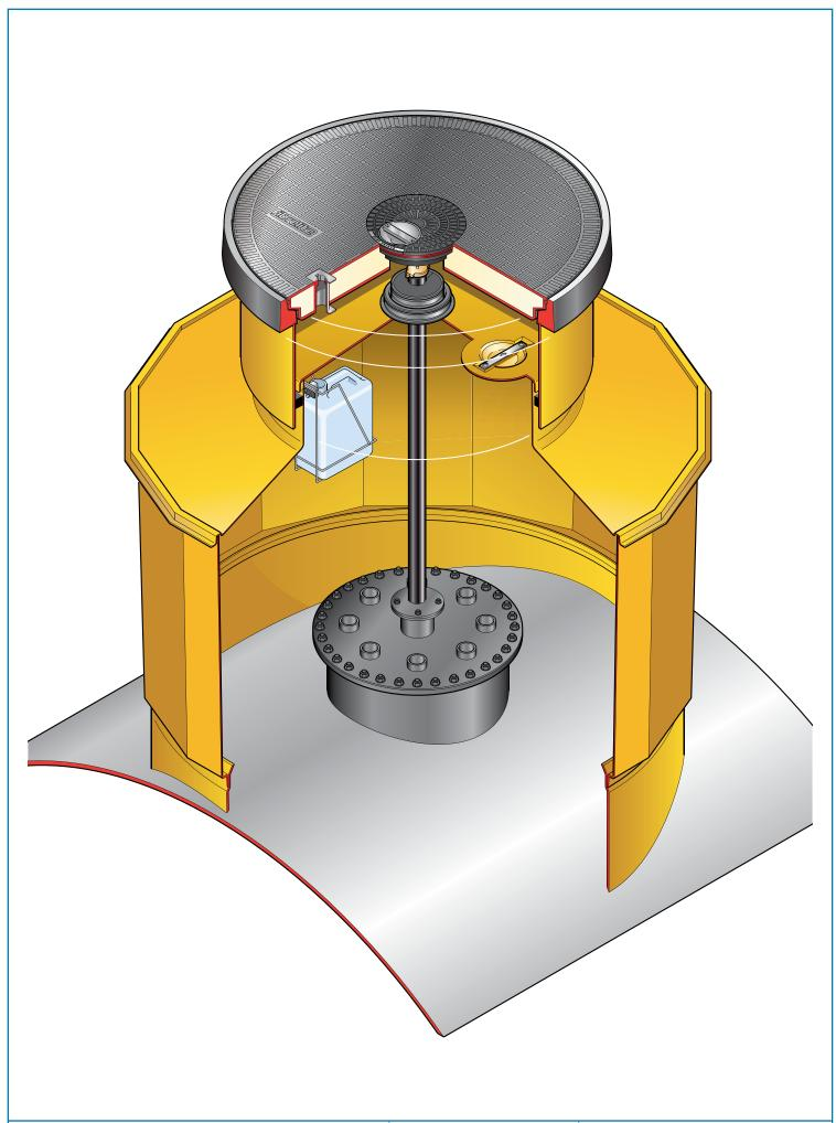
1.7m diameter stackable sump with collar ring base, stackable corbel, non-structural internal lid, adjustable height skirt, round 1020mm flat sealed cover and frame.
