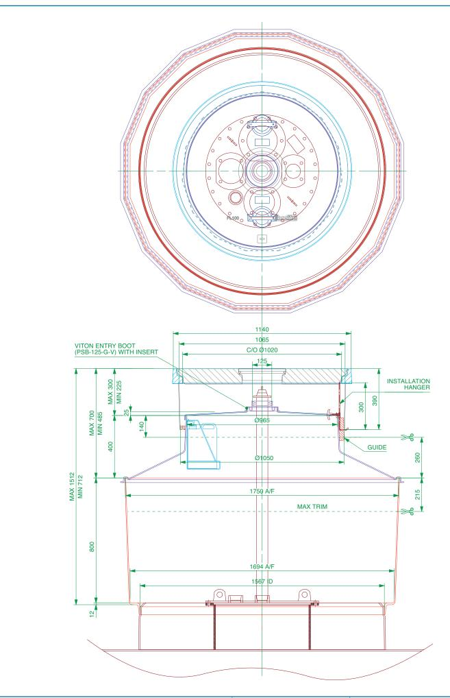
1.7m diameter stackable sump with collar ring base, stackable corbel, non-structural internal lid, adjustable height skirt, round 1020mm flat sealed cover and frame.
