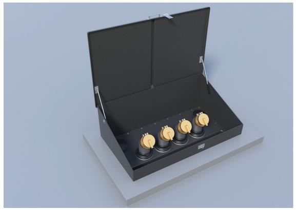
1237 mm x 686 mm x 1257 mm deep GRP above ground fill sump with hinged door to fit up to 4 fill lines. System includes internal spill tray, pipework support rail and concrete tie fixings.
