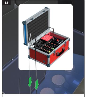
Connect the vacuum hoses to the plate and commence test. The test module must only be set to a depth setting of 0.6m.
