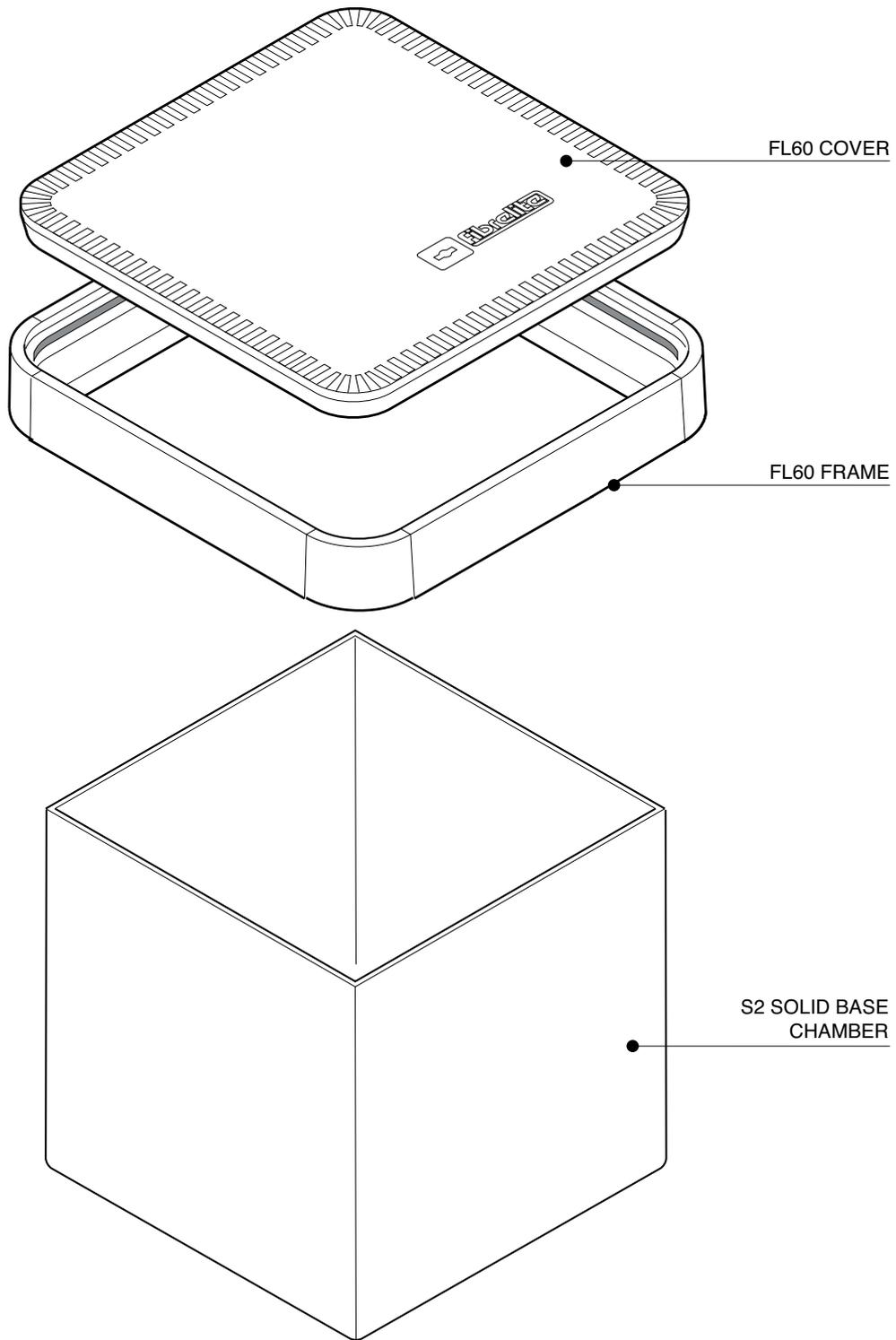
600mm square x 600mm deep solid base chamber with a square 600mm flat sealed cover.
