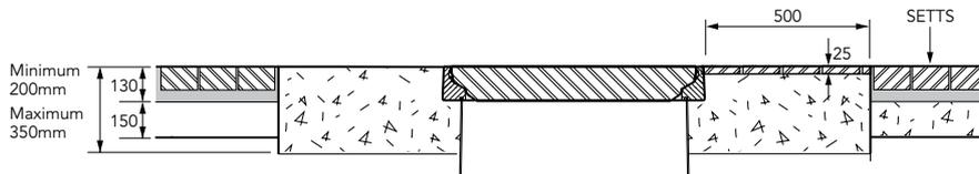
600mm square x 600mm deep solid base chamber with a square 600mm flat sealed cover.
