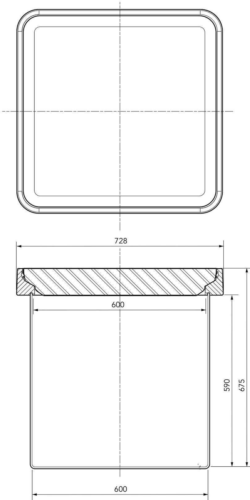
600mm square x 600mm deep solid base chamber with a square 600mm flat sealed cover.
