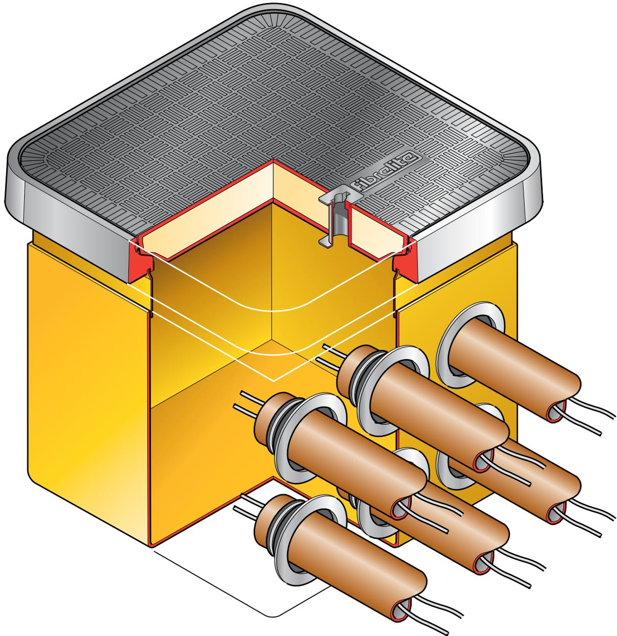
Electrical Drawpit - 600mm cubed GRP chamber with a 110mm deep skirt, 600mm square flat sealed cover and frame.
