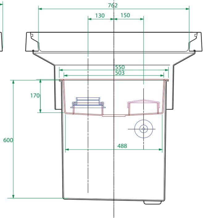
500mm square x 600mm deep GRP solid base sump, GRP spill container, GRP skirt, 760mm dia flat sealed cover and frame. 1/2 tin sealant. Designed to fit Environ pipework. 2 Fills.
