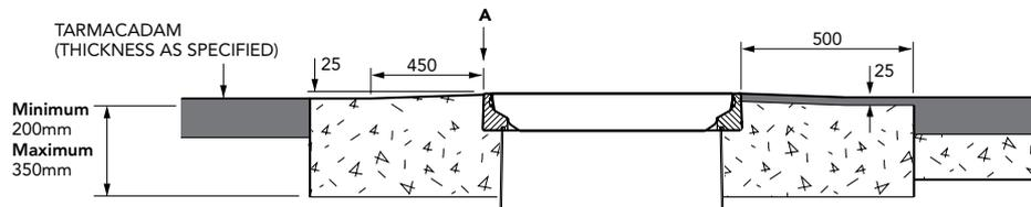
500mm square x 600mm deep GRP solid base sump, GRP spill container, GRP skirt, 760mm dia flat sealed cover and frame. ½ tin sealant. Designed to fit Environ pipework. 2 Fills.
