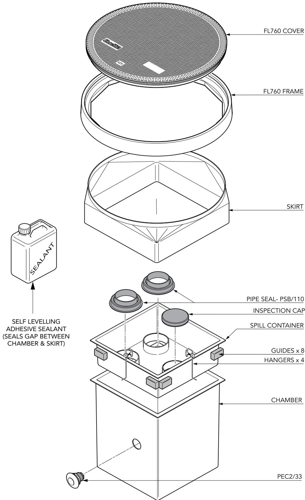
500mm square x 600mm deep GRP solid base sump, GRP spill container, GRP skirt, 760mm dia flat sealed cover and frame. ½ tin sealant. Designed to fit Environ pipework. 2 Fills.
