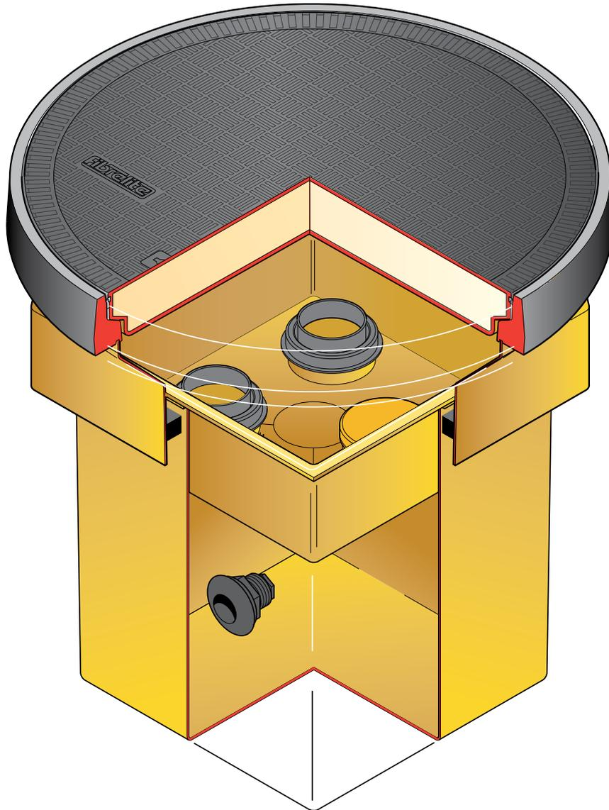
500mm square x 600mm deep GRP solid base sump, GRP spill container, GRP skirt, 760mm dia flat sealed cover and frame. ½ tin sealant. Designed to fit Environ pipework. 2 Fills.
