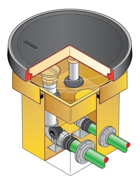
500mm square x 600mm deep GRP solid base sump, GRP spill container, GRP skirt, 760mm dia flat sealed cover and frame.  $\frac{1}{2}$  tin sealant. Designed to fit Environ pipework. 1 Fill and 1 VR1B
