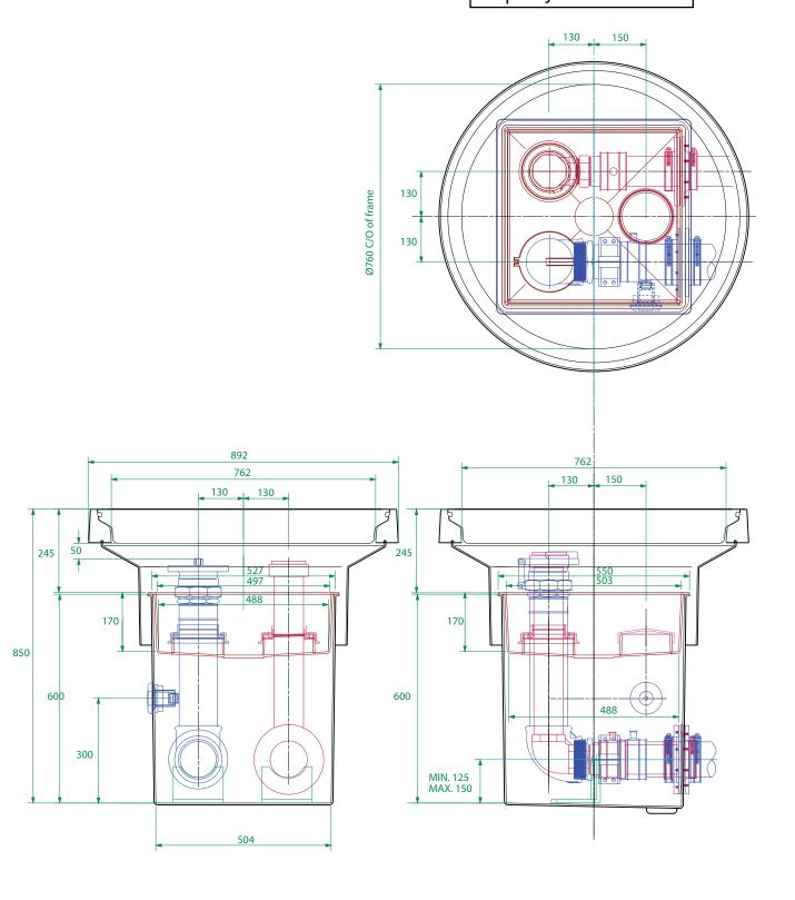
500mm square x 600mm deep GRP solid base sump, GRP spill container, GRP skirt, 760mm dia flat sealed cover and frame.  $\frac{1}{2}$  tin sealant. Designed to fit Environ pipework. 1 Fill and 1 VR1B
