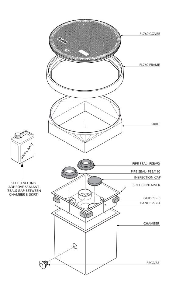
500mm square x 600mm deep GRP solid base sump, GRP spill container, GRP skirt, 760mm dia flat sealed cover and frame.  $\frac{1}{2}$  tin sealant. Designed to fit Environ pipework. 1 Fill and 1 VR1B
