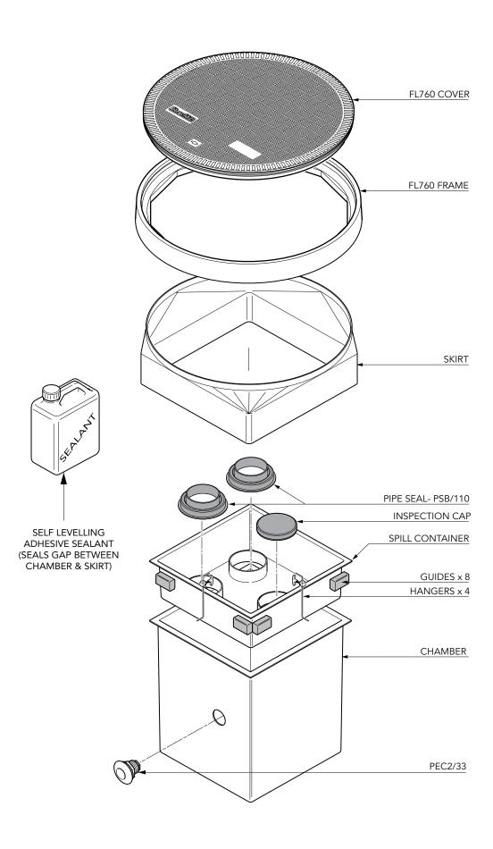
500mm square x 600mm deep GRP solid base sump, GRP spill container, GRP skirt, 760mm dia flat sealed cover and frame.  $\frac{1}{2}$  tin sealant. Designed to fit Environ pipework. 2 Fills.
