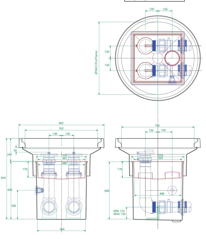
500mm square x 600mm deep GRP solid base sump, GRP spill container, GRP skirt, 760mm dia flat sealed cover and frame.  $\frac{1}{2}$  tin sealant. Designed to fit Environ pipework. 2 Fills.
