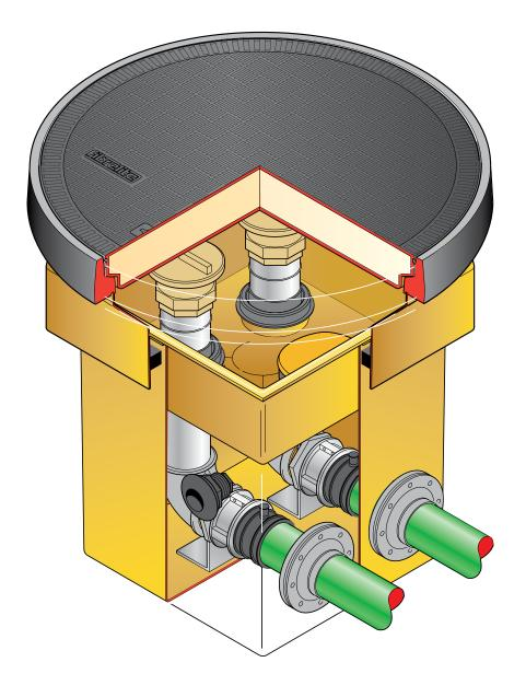
500mm square x 600mm deep GRP solid base sump, GRP spill container, GRP skirt, 760mm dia flat sealed cover and frame.  $\frac{1}{2}$  tin sealant. Designed to fit Environ pipework. 2 Fills.
