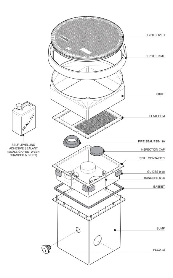
490mm square x 600mm deep offset fill chamber system with adjustable skirt, spill container, platfrom, 1/2 tin of sealant and FL760 flat sealed cover with composite frame. Includes inspection port cap, pipe entry and penetration fitting for grounding connection. Includes preinstalled KPS pipework for 1 fill.
