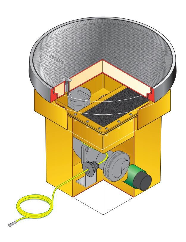
490mm square x 600mm deep offset fill chamber system with adjustable skirt, spill container, platfrom, 1/2 tin of sealant and FL760 flat sealed cover with composite frame. Includes inspection port cap, pipe entry and penetration fitting for grounding connection. Includes preinstalled KPS pipework for 1 fill.
