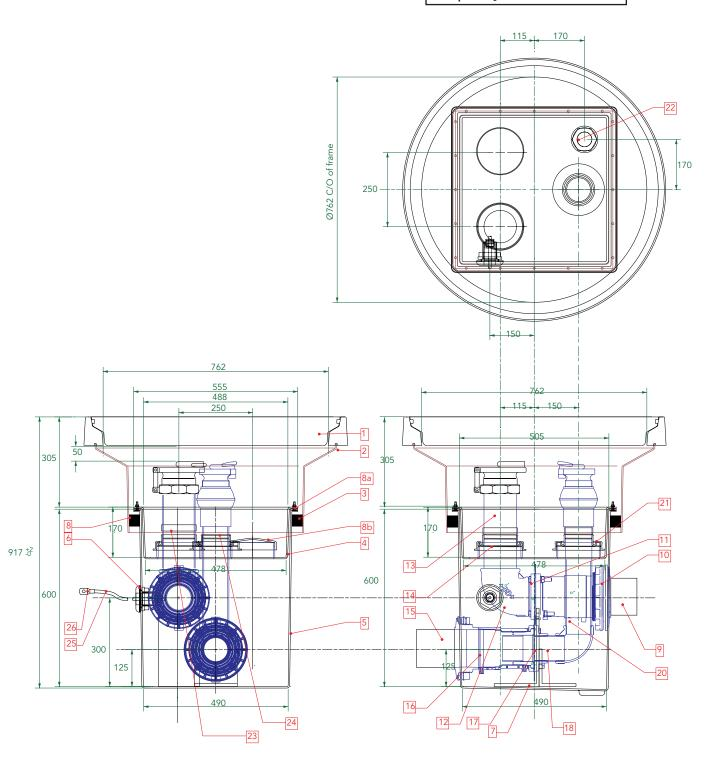
$490 mm \, x \, 600 mm$  GRP chamber with a GRP spill container and 762mm diameter round flat sealed cover. 1 x Fill & 1 VR
