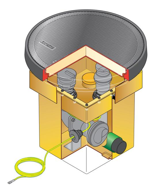
$490 mm \, x \, 600 mm$  GRP chamber with a GRP spill container and 762mm diameter round flat sealed cover. 1 x Fill & 1 VR
