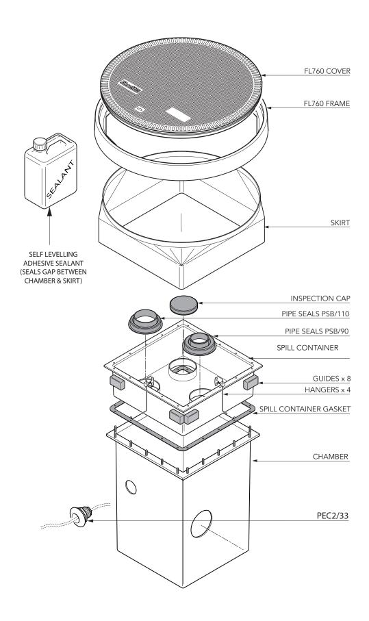
$490 mm \, x \, 600 mm$  GRP chamber with a GRP spill container and 762mm diameter round flat sealed cover. 1 x Fill & 1 VR
