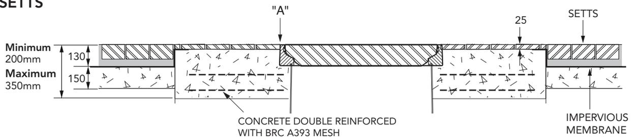
490mm square x 600mm deep offset fill chamber system with adjustable skirt, spill container, platform, 1/2 tin of sealant and FL760 flat sealed cover with composite frame. Includes inspection port cap, pipe entry and penetration fitting for grounding connection. Includes preinstalled KPS pipework for 2 fills.
