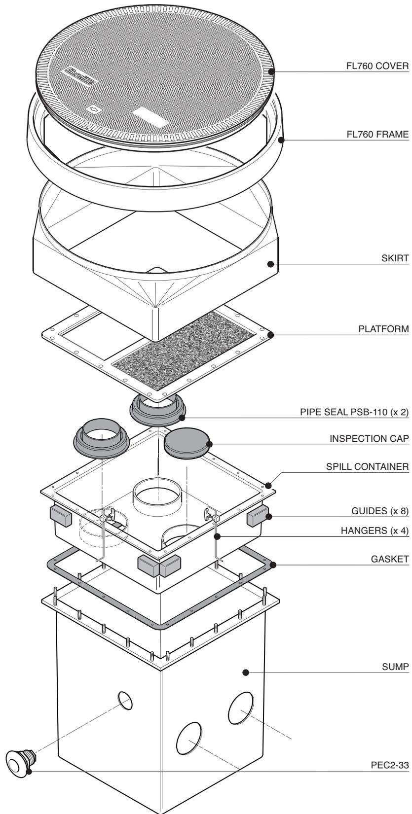
490mm square x 600mm deep offset fill chamber system with adjustable skirt, spill container, platform, 1/2 tin of sealant and FL760 flat sealed cover with composite frame. Includes inspection port cap, pipe entry and penetration fitting for grounding connection. Includes preinstalled KPS pipework for 2 fills.
