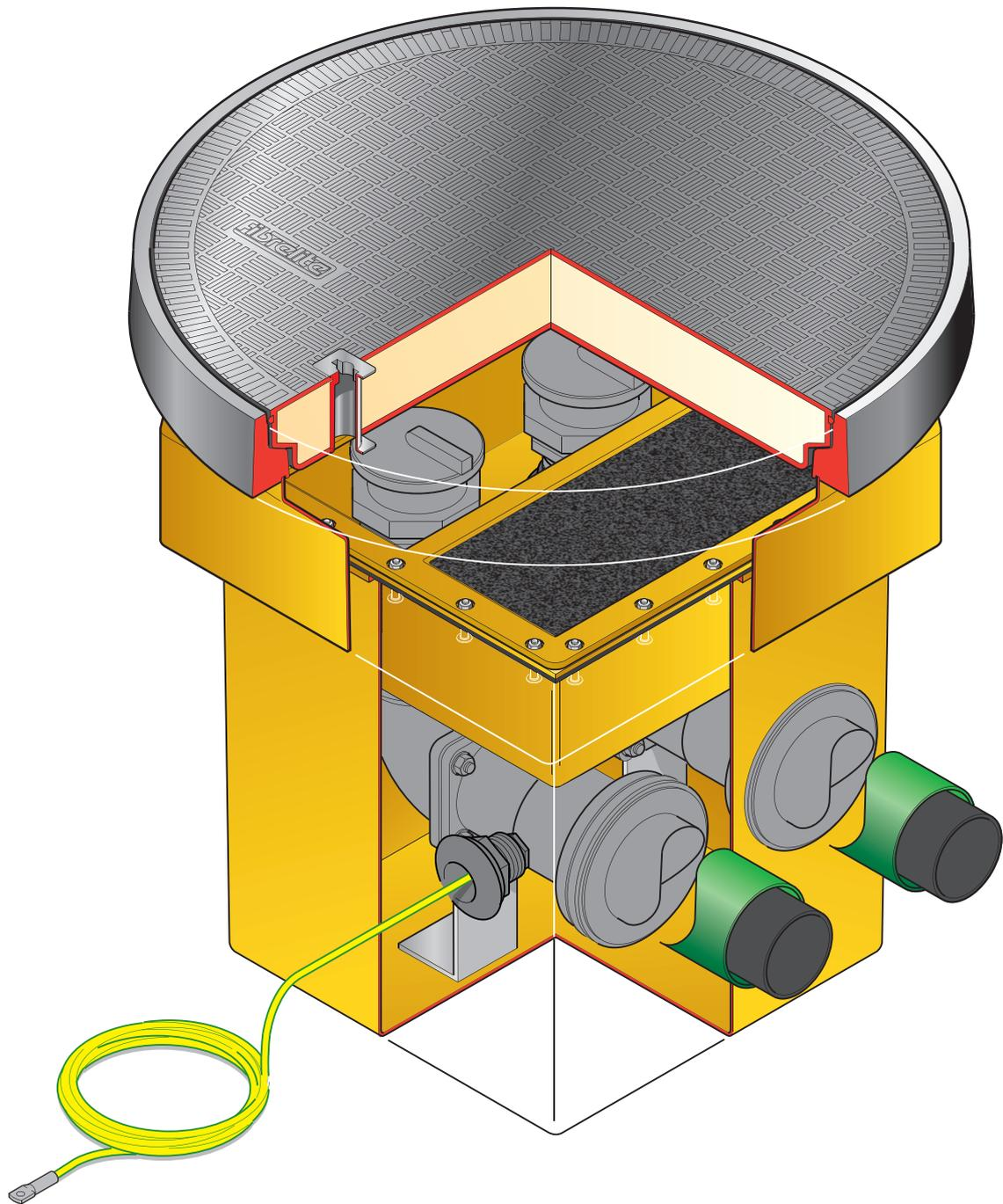
490mm square x 600mm deep offset fill chamber system with adjustable skirt, spill container, platform, 1/2 tin of sealant and FL760 flat sealed cover with composite frame. Includes inspection port cap, pipe entry and penetration fitting for grounding connection. Includes preinstalled KPS pipework for 2 fills.
