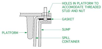
Structural platform to fit S2-360/OF & S2-3760/OF chamber systems. Includes letterbox style hole and anti-slip surface. Designed to fit bolted spill trays.
