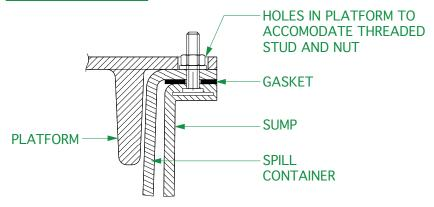
Solid structural platform to fit S2-360/OF & S2-3760/OF chamber systems. Includes anti-slip surface.
