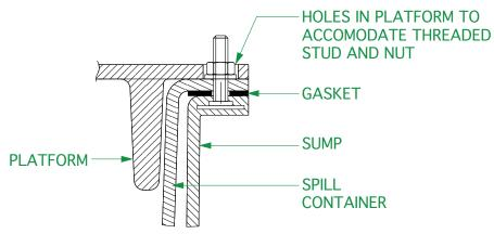
Structural platform to fit S2-360/OF & S2-3760/OF chamber systems. Includes one or two 195mm dia. holes and anti slip surface. Specify hole requirement when ordering. Designed to fit bolted spill trays.
