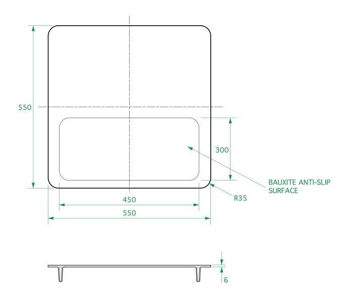
Solid structural platform to fit S2-360/OF & S2-3760/OF chamber systems. Includes anti slip surface.
