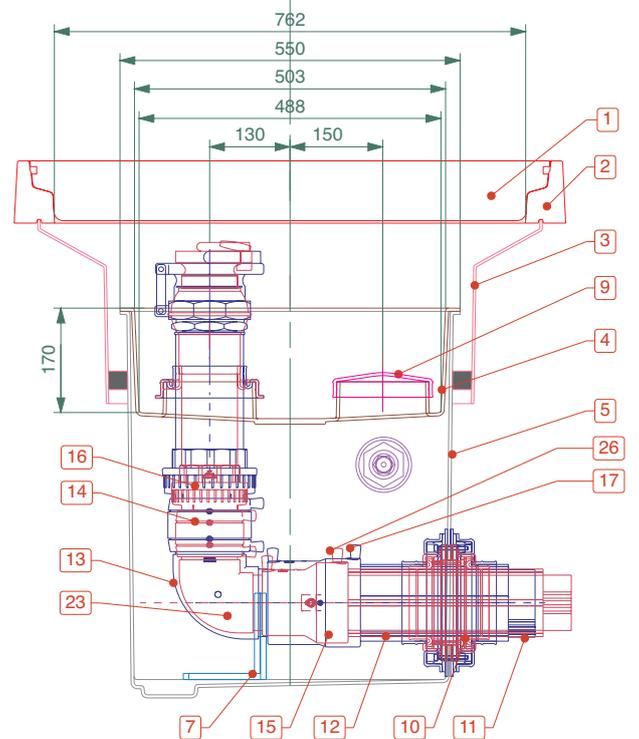
500mm square x 600mm deep GRP solid base sump, GRP spill container, GRP skirt, 760mm dia flat sealed cover and frame. ½ tin sealant. Designed to fit UPP pipework. 1 Fill and VR1b.
