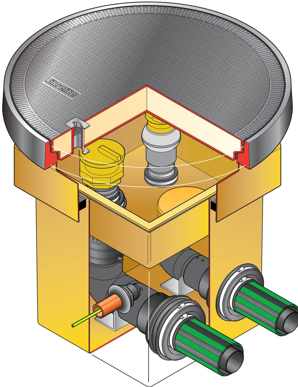
500mm square x 600mm deep GRP solid base sump, GRP spill container, GRP skirt, 760mm dia flat sealed cover and frame. ½ tin sealant. Designed to fit UPP pipework. 1 Fill and VR1b.
