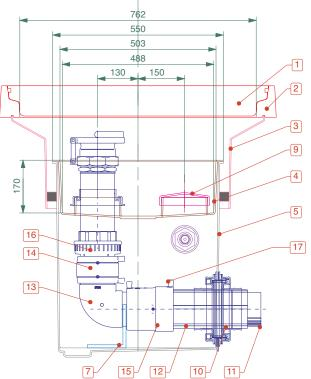
500mm square x 600mm deep GRP solid base sump, GRP spill container, GRP skirt, 760mm dia flat sealed cover and frame.  $\frac{1}{2}$  tin sealant. Designed to fit UPP pipework. 2 Fills
