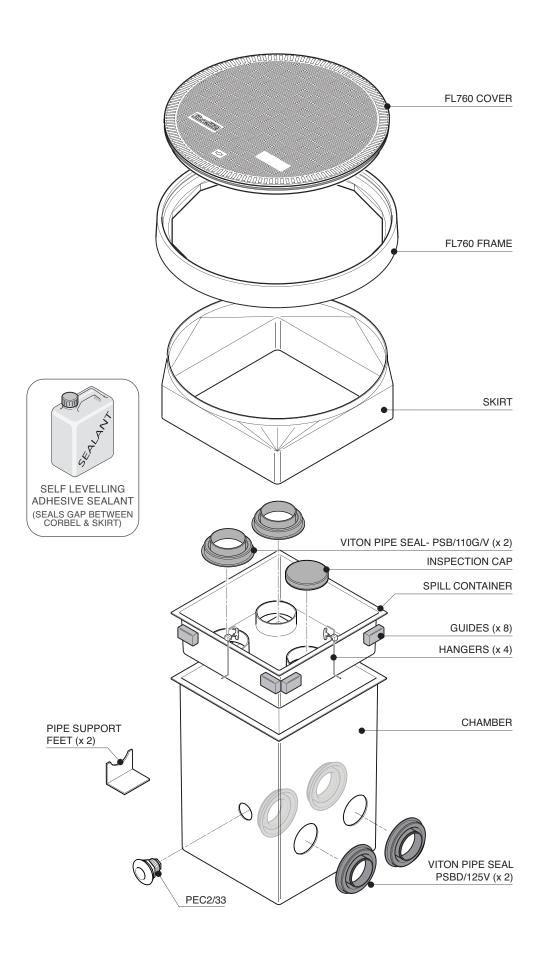
500mm square x 600mm deep GRP solid base sump, GRP spill container, GRP skirt, 760mm dia flat sealed cover and frame.  $\frac{1}{2}$  tin sealant. Designed to fit UPP pipework. 2 Fills
