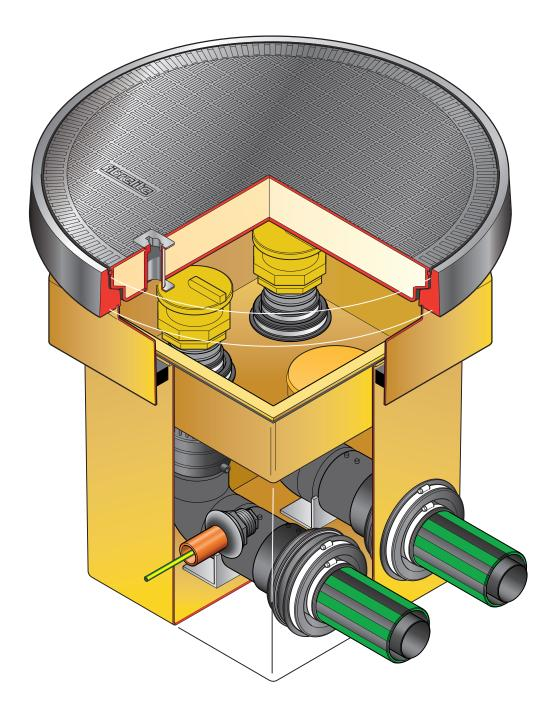
500mm square x 600mm deep GRP solid base sump, GRP spill container, GRP skirt, 760mm dia flat sealed cover and frame.  $\frac{1}{2}$  tin sealant. Designed to fit UPP pipework. 2 Fills
