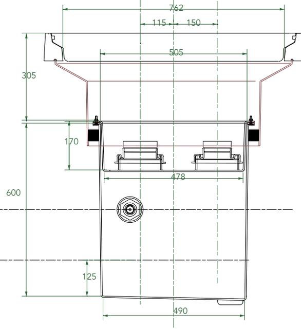
490mm x 600mm GRP chamber with a GRP spill container with an intergrated drainback system and 762mm diameter round flat sealed cover.
