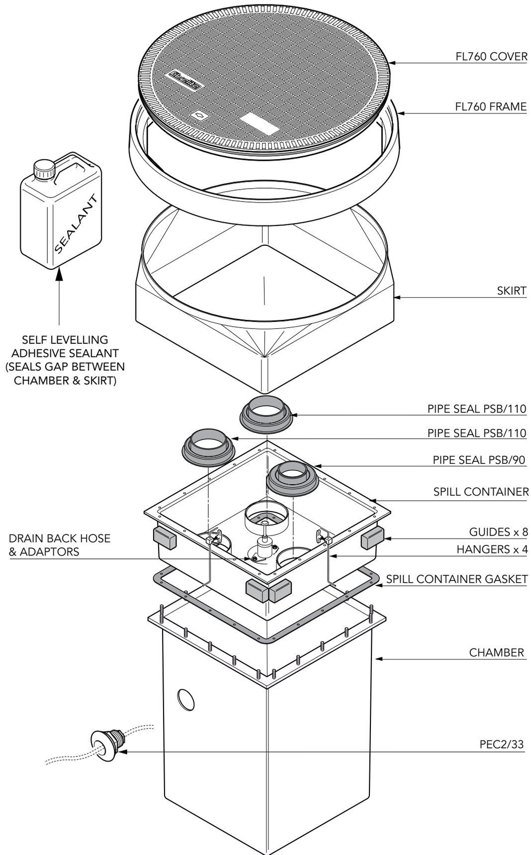
490mm x 600mm GRP chamber with a GRP spill container with an intergrated drainback system and 762mm diameter round flat sealed cover.
