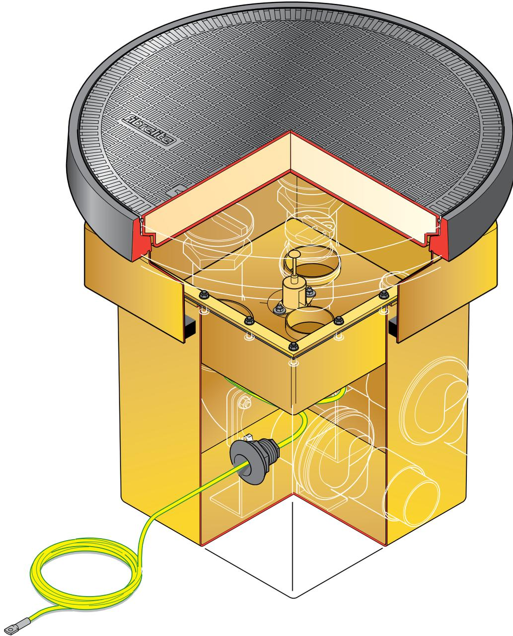
490mm x 600mm GRP chamber with a GRP spill container with an intergrated drainback system and 762mm diameter round flat sealed cover.
