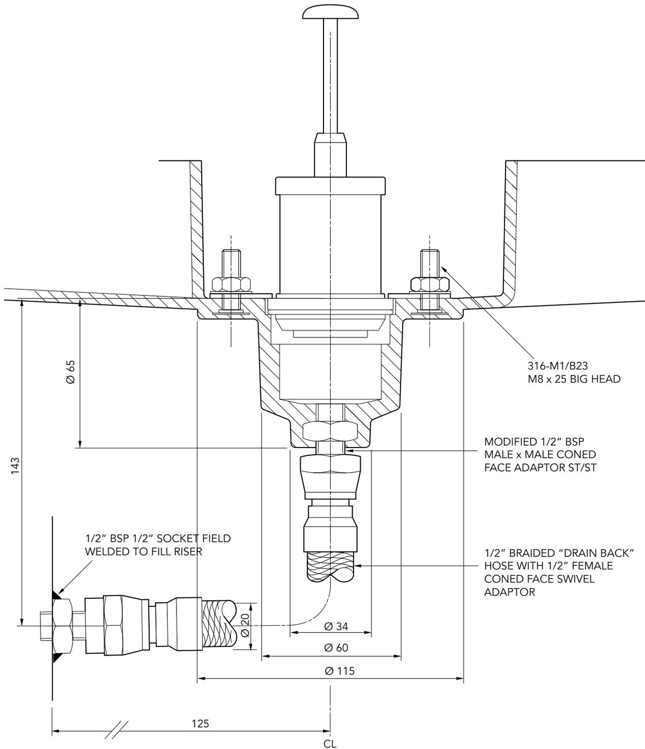
500mm square x 600mm deep GRP solid base sump. GRP spill container with an integrated drainback system, GRP skirt, 760mm dia flat sealed cover and frame. Designed to fit Environ pipework. 1 Fill and 1 VR1B
