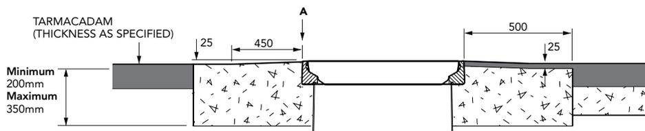
500mm square x 600mm deep GRP solid base sump, GRP spill container with an integrated drainback system, GRP skirt, 760mm dia flat sealed cover and frame. Designed to fit Environ pipework. 1 Fill and 1 VR1B
