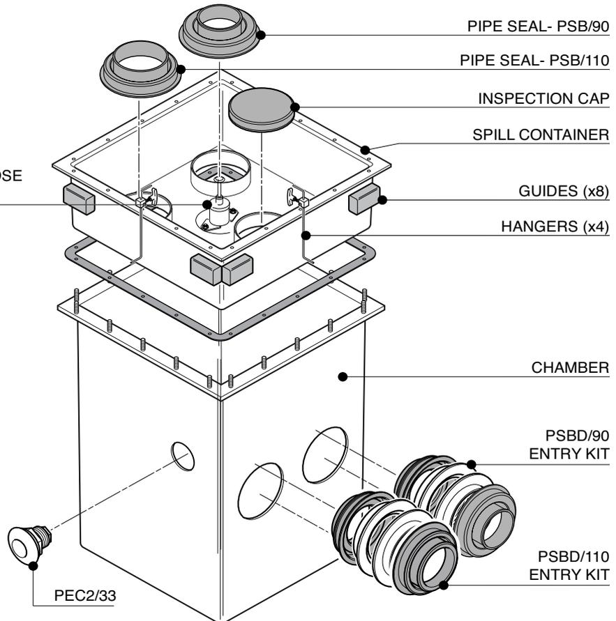
500mm square x 600mm deep GRP solid base sump. GRP spill container with an integrated drainback system, GRP skirt, 760mm dia flat sealed cover and frame. Designed to fit Environ pipework. 1 Fill and 1 VR1B
