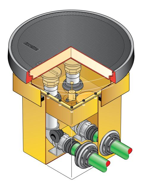
500mm square x 600mm deep GRP solid base sump, GRP spill container with an integrated drainback system, GRP skirt, 760mm dia flat sealed cover and frame.  $\frac{1}{2}$  tin sealant. Designed to fit Environ pipework. 2 Fills.
