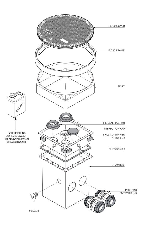
500mm square x 600mm deep GRP solid base sump, GRP spill container with an integrated drainback system, GRP skirt, 760mm dia flat sealed cover and frame. % tin sealant. Designed to fit Environ pipework. 2 Fills.
