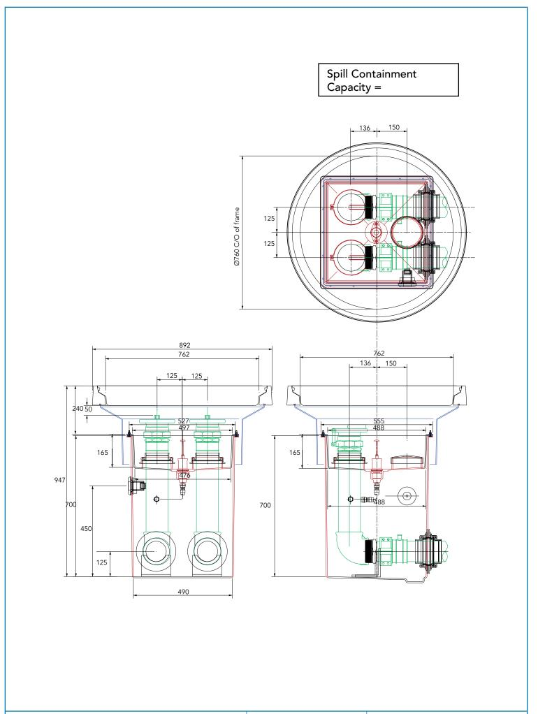
500mm square x 600mm deep GRP solid base sump, GRP spill container with an integrated drainback system, GRP skirt, 760mm dia flat sealed cover and frame. % tin sealant. Designed to fit Environ pipework. 2 Fills.
