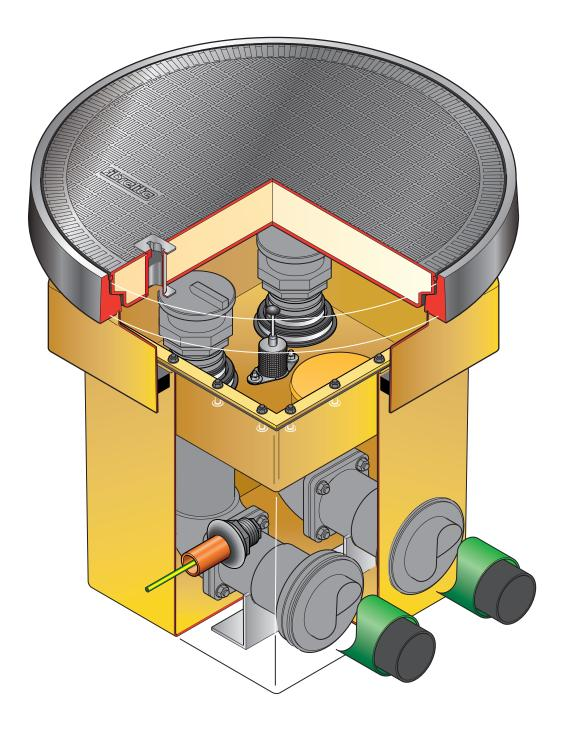
490mm square x 770mm deep offset fill chamber system with adjustable skirt, integrated spill container with intergrated drainback, 1/2 tin of sealant and FL760 flat sealed cover with composite frame. Includes inspection port cap, pipe entry and penetration fitting for grounding connection. Includes preinstalled KPS pipework for 2 fills.
