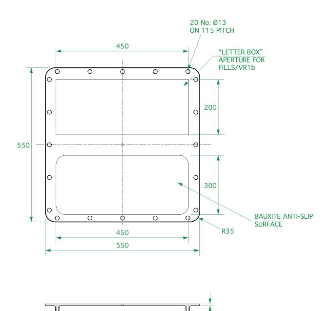
Structural platform to fit S2-360/OFD & S2-3760/OFD chamber systems. Includes letterbox style hole, anti-slip surface and a hole to fit a drainback valve plunger. Designed to fit bolted spill trays.
