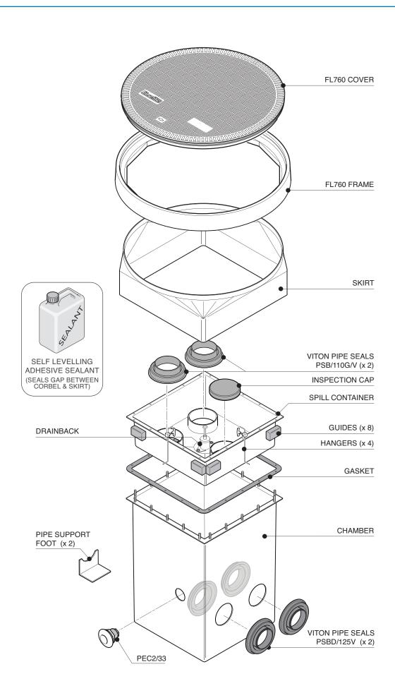
500mm square x 600mm deep GRP solid base sump, GRP spill container with an integrated drainback system, GRP skirt, 760mm dia flat sealed cover and frame.  $\frac{1}{2}$  tin sealant. Designed to fit UPP pipework. 2 Fills.
