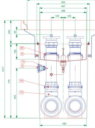
500mm square x 600mm deep GRP solid base sump, GRP spill container with an integrated drainback system, GRP skirt, 760mm dia flat sealed cover and frame.  $\frac{1}{2}$  tin sealant. Designed to fit UPP pipework. 2 Fills.
