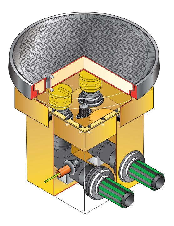
500mm square x 600mm deep GRP solid base sump, GRP spill container with an integrated drainback system, GRP skirt, 760mm dia flat sealed cover and frame.  $\frac{1}{2}$  tin sealant. Designed to fit UPP pipework. 2 Fills.
