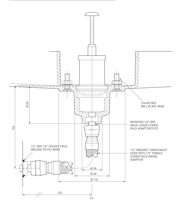
500mm square x 600mm deep GRP solid base sump, GRP spill container with an integrated drainback system, GRP skirt, 760mm dia flat sealed cover and frame.  $\frac{1}{2}$  tin sealant. Designed to fit UPP pipework. 2 Fills.
