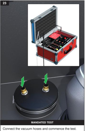
Connect the vacuum hoses and commence the test. The test module must only be set to a depth setting of 0.6m.
