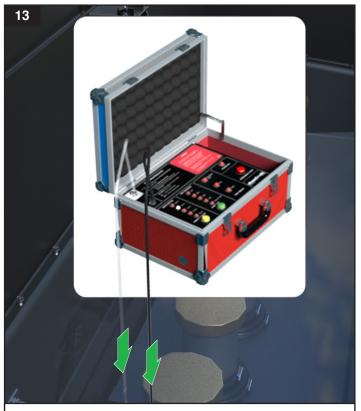
Connect the vacuum hoses to the plate and commence test. The test module must only be set to a depth setting of 0.6m.
