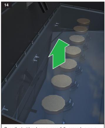
Once the test has been successfully passed, remove the spill container and pipe plugs.
