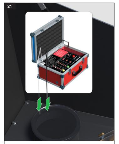
Connect the vacuum hoses and commence the test. The test module must only be set to a depth setting of 0.6m.
