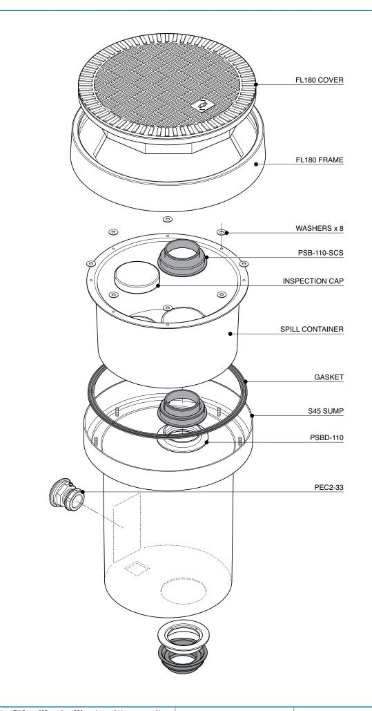
Secondary Contained Direct Fill Sump 385mm dia. x 550mm deep solid base sump, with a sealed secondary spill container and integrated drainback valve system. 450mm dia. flat sealed cover and frame. Includes PSBD-110-SCS 110mm dia fill pipe sealkit and grounding cable sealkit. Direct Fill not suitable for stage 1 co-axial vapour recovery
