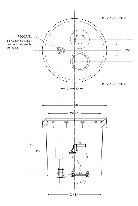
DOUBLE TANK RISER GROUNDBOX 485mm dia. x 450mm deep solid base sump with a 457mm dia flat sealed grey cover and frame. Designed to contain two tank risers & two conduits. Entry kits to be ordered separately
