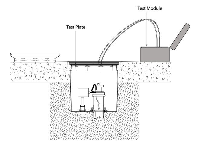
DOUBLE TANK RISER GROUNDBOX 485mm dia. x 450mm deep solid base sump with a 457mm dia flat sealed grey cover and frame. Designed to contain two tank risers & two conduits. Entry kits to be ordered separately
