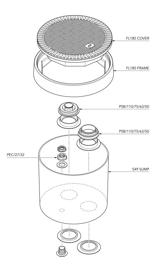
DOUBLE TANK RISER GROUNDBOX 485mm dia. x 450mm deep solid base sump with a 457mm dia flat sealed grey cover and frame. Designed to contain two tank risers & two conduits. Entry kits to be ordered separately
