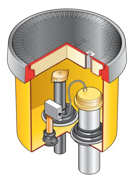
DOUBLE TANK RISER GROUNDBOX 485mm dia. x 450mm deep solid base sump with a 457mm dia flat sealed grey cover and frame. Designed to contain two tank risers & two conduits. Entry kits to be ordered separately
