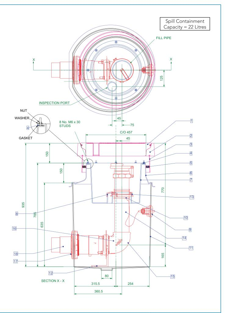
Secondary contained remote fill sump. 570mm dia. x 635mm deep solid base sump with a sealed secondary spill container. 450mm dia flat sealed cover and frame. Includes PEC2/33 grounding sealkit and pre-fitted KPS 125/110 secondary contained
