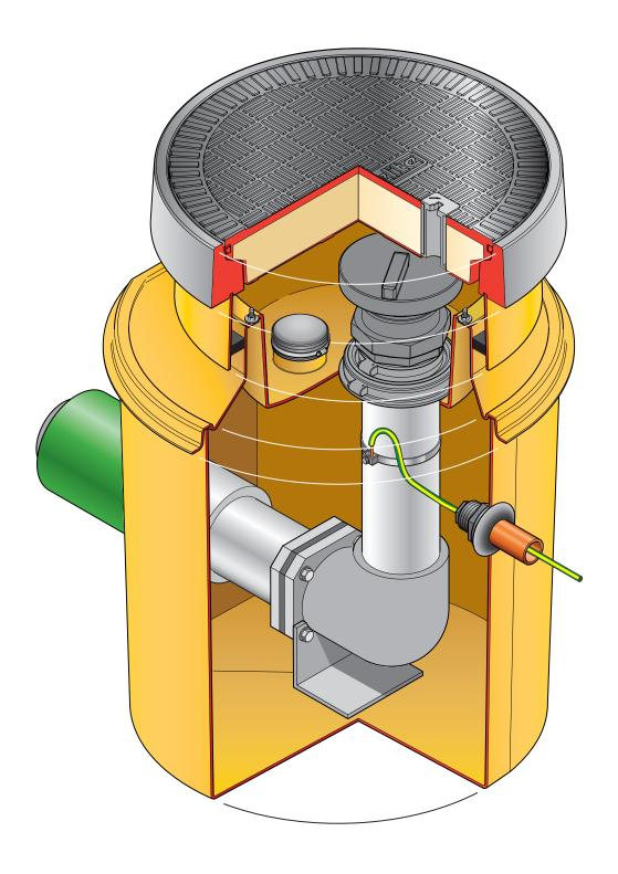
Secondary contained remote fill sump. 570mm dia. x 635mm deep solid base sump with a sealed secondary spill container. 450mm dia flat sealed cover and frame. Includes PEC2/33 grounding sealkit and pre-fitted KPS 125/110 secondary contained pipework.
