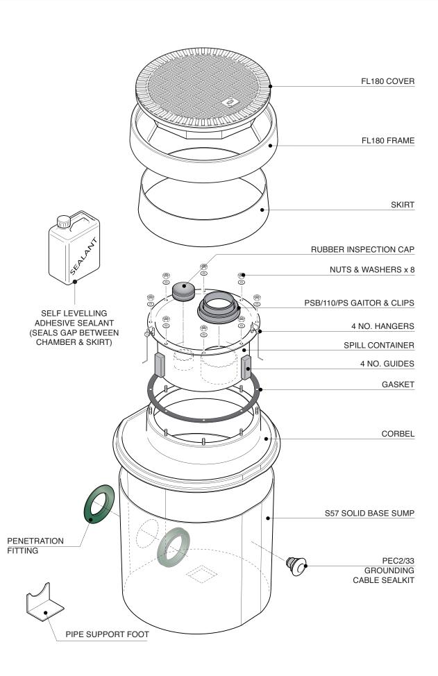
Secondary contained remote fill sump. 570mm dia. x 635mm deep solid base sump with a sealed secondary spill container. 450mm dia flat sealed cover and frame. Includes PEC2/33 grounding sealkit and pre-fitted KPS 125/110 secondary contained
