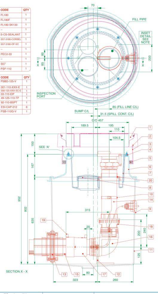
Secondary contained remote fill sump. 583mm dia. x 635mm deep solid base sump with a sealed secondary spill container. 450mm dia flat sealed cover and frame. Sealkits included.
