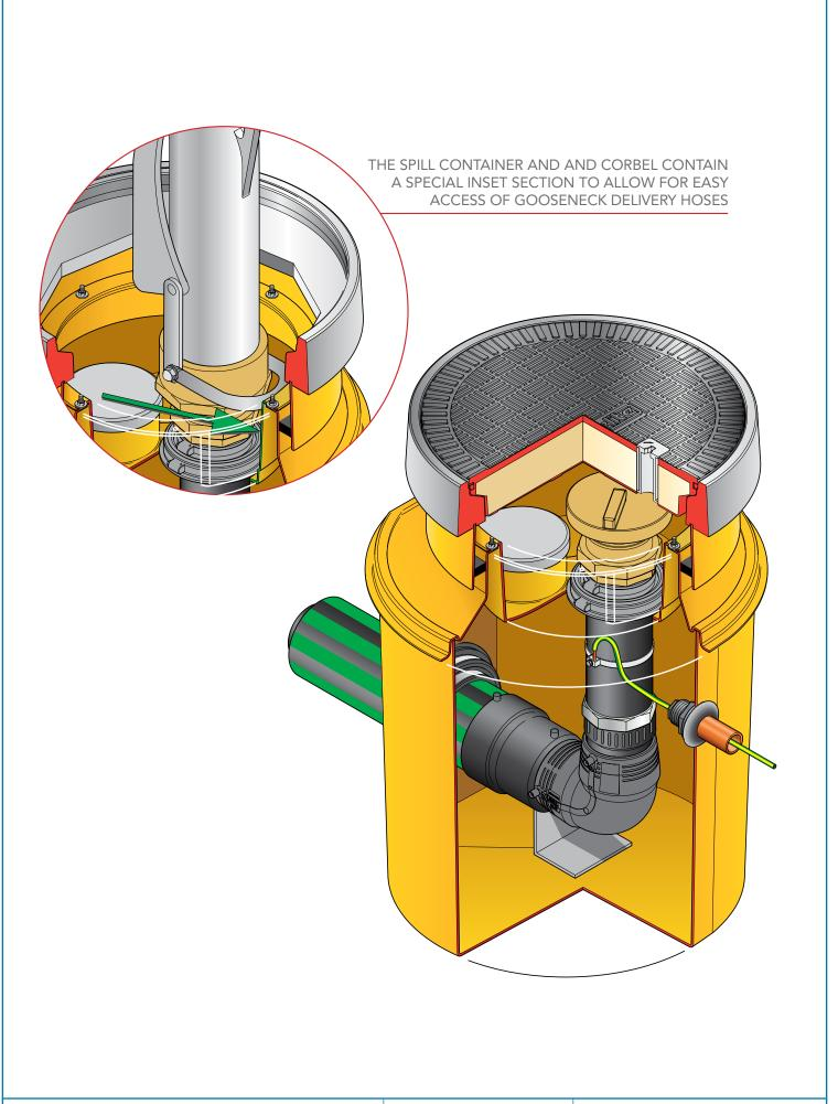
Secondary contained remote fill sump. 583mm dia. x 635mm deep solid base sump with a sealed secondary spill container. 450mm dia flat sealed cover and frame. Sealkits included.
