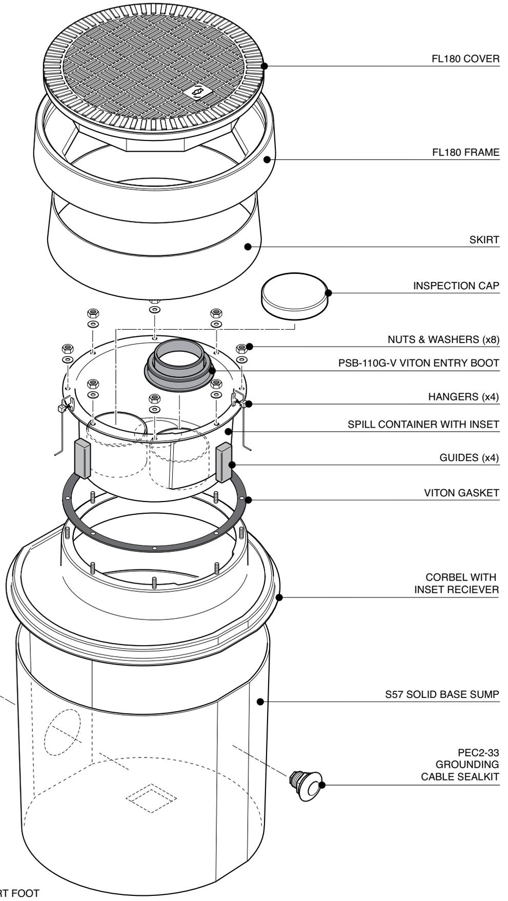
Secondary contained remote fill sump. 583mm dia. x 635mm deep solid base sump and a sealed secondary spill container. 450mm dia flat sealed cover and frame. Includes PSB-110-PS 110mm dia. spill tray fill riser sealkit and grounding cable sealkit.
