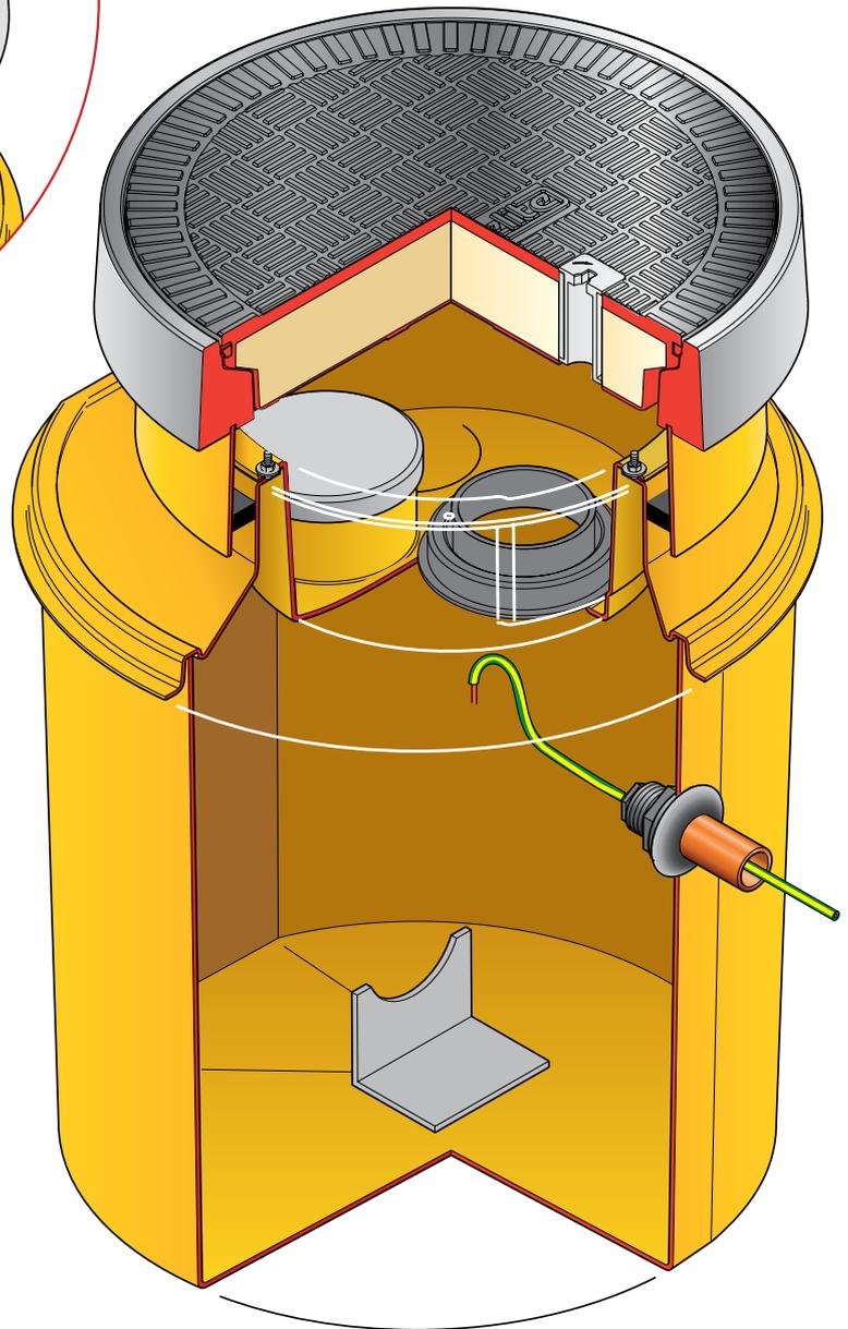
Secondary contained remote fill sump. 583mm dia. x 635mm deep solid base sump and a sealed secondary spill container. 450mm dia flat sealed cover and frame. Includes PSB-110-PS 110mm dia. spill tray fill riser sealkit and grounding cable sealkit.
