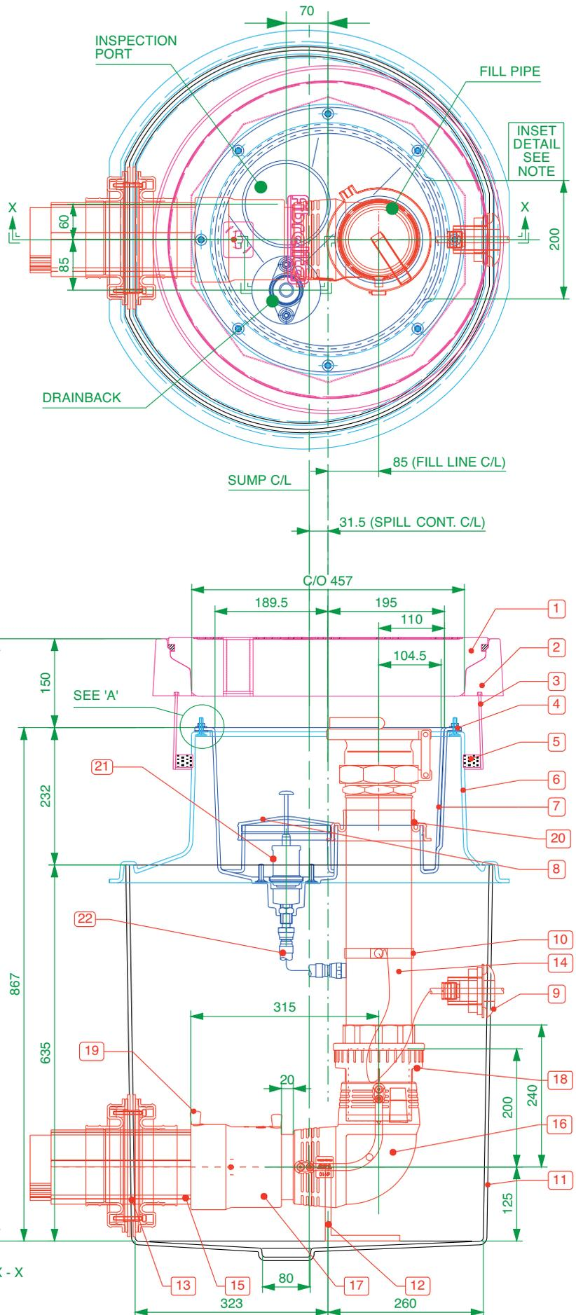
Secondary contained remote fill sump. 583mm dia. x 635mm deep solid base sump with a sealed secondary spill container with integrated drainback system. 450mm dia flat sealed cover and frame. Sealkits included.
