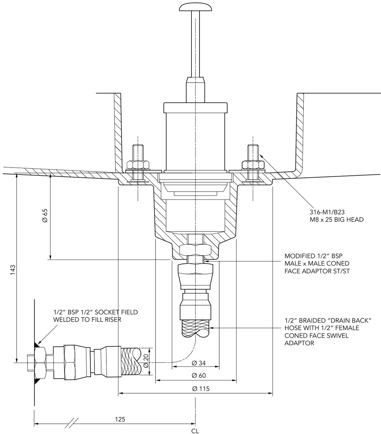
Secondary contained remote fill sump. 583mm dia. x 635mm deep solid base sump with a sealed secondary spill container with integrated drainback system. 450mm dia flat sealed cover and frame. Sealkits included.
