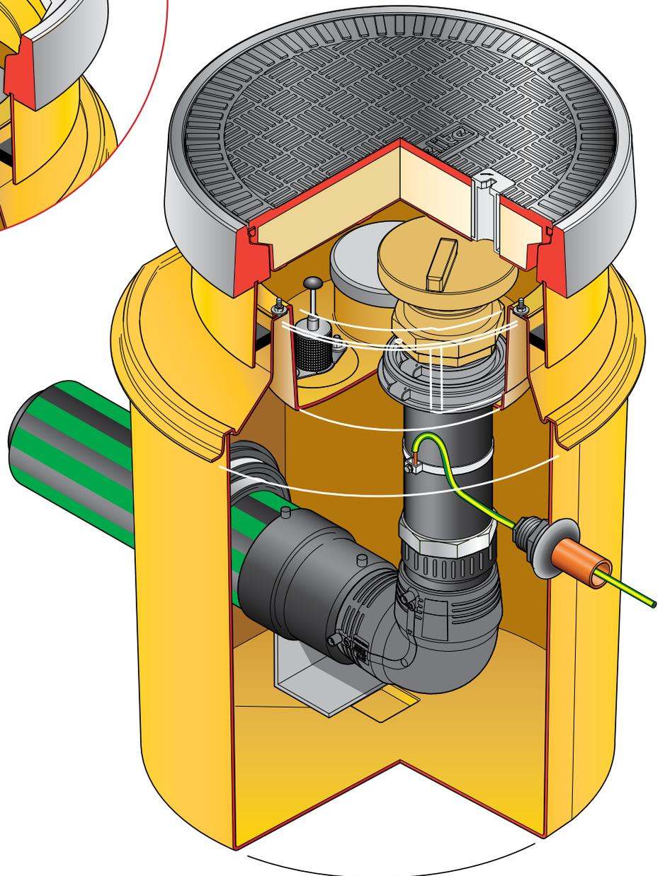
Secondary contained remote fill sump. 583mm dia. x 635mm deep solid base sump with a sealed secondary spill container with integrated drainback system. 450mm dia flat sealed cover and frame. Sealkits included.
