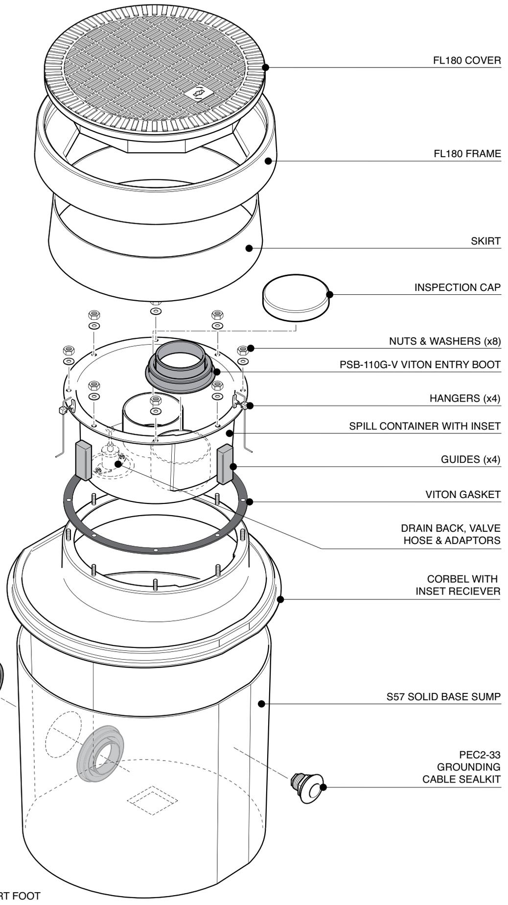
Secondary contained remote fill sump. 583mm dia. x 635mm deep solid base sump with a sealed secondary spill container with integrated drainback system. 450mm dia flat sealed cover and frame. Sealkits included.
