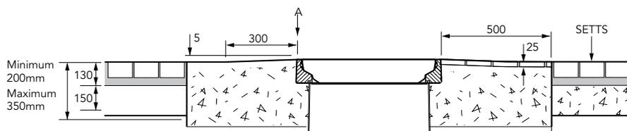
Secondary contained remote fill sump. 583mm dia. x 635mm deep solid base sump with a sealed secondary spill container with integrated drainback system. 450mm dia flat sealed cover and frame. Sealkits included.
