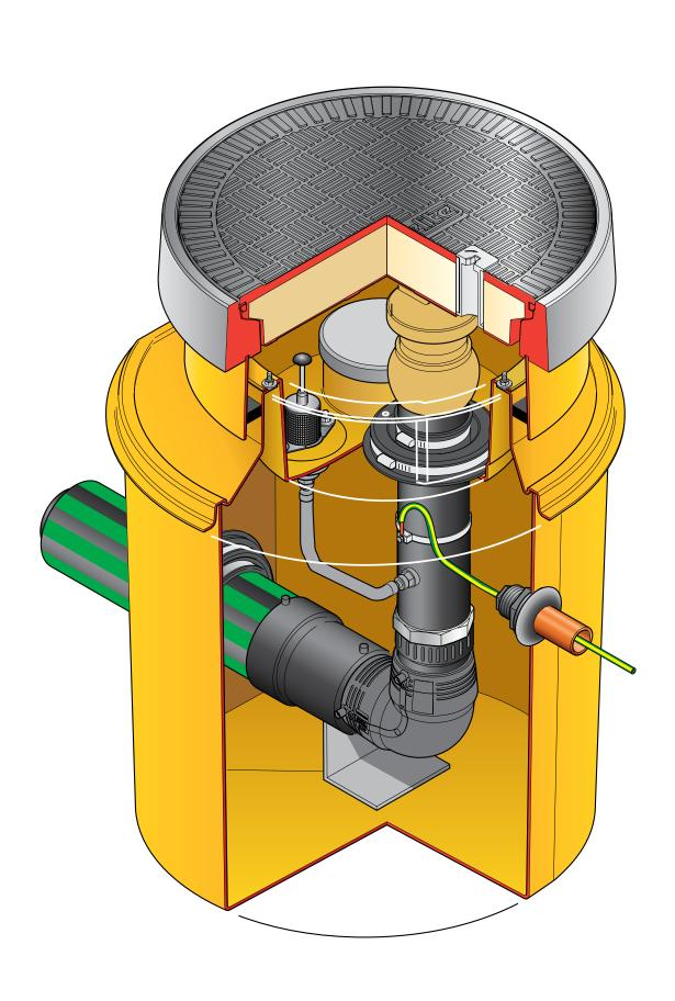
Secondary contained vapour recovery sump. 570mm dia. x 635mm deep solid base sump with a sealed secondary spill container and integrated drainback system. 450mm dia flat sealed cover and frame. Pipework included.
