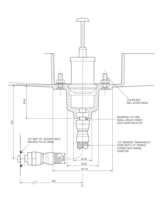
Secondary contained vapour recovery sump. 570mm dia. x 635mm deep solid base sump with a sealed secondary spill container and integrated drainback system. 450mm dia flat sealed cover and frame. Pipework included.
