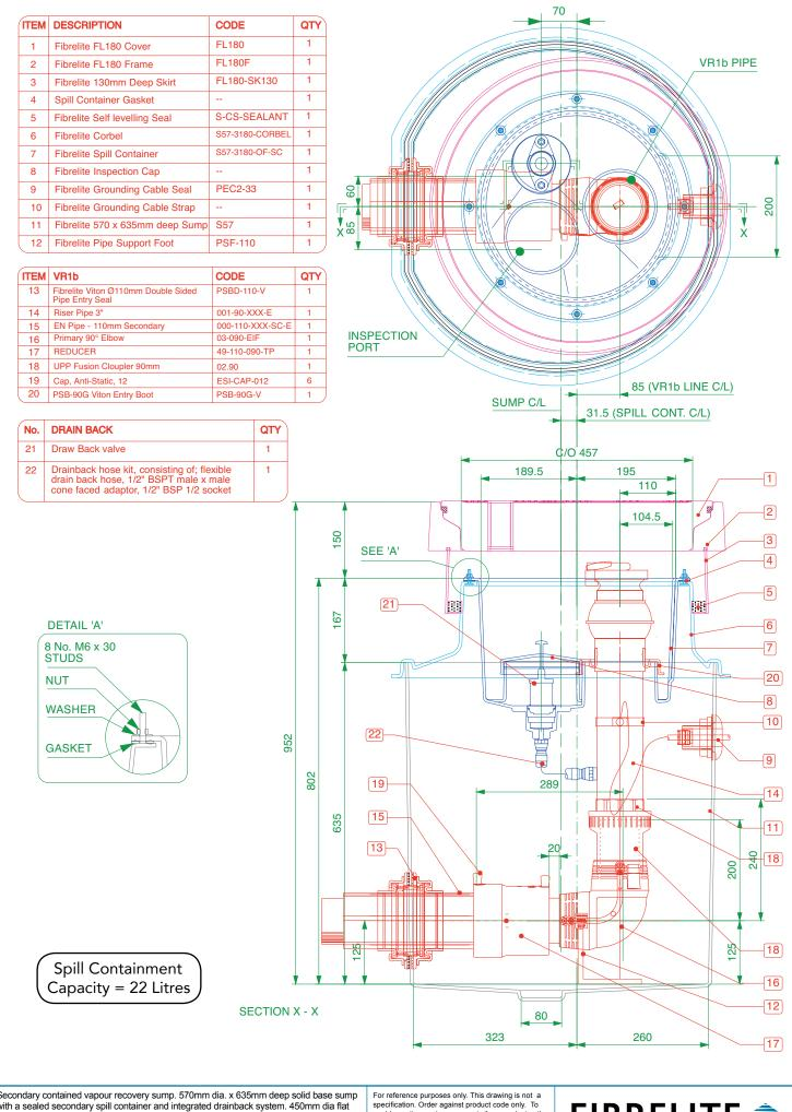
Secondary contained vapour recovery sump. 570mm dia. x 635mm deep solid base sump with a sealed secondary spill container and integrated drainback system. 450mm dia flat sealed cover and frame. Pipework included.
