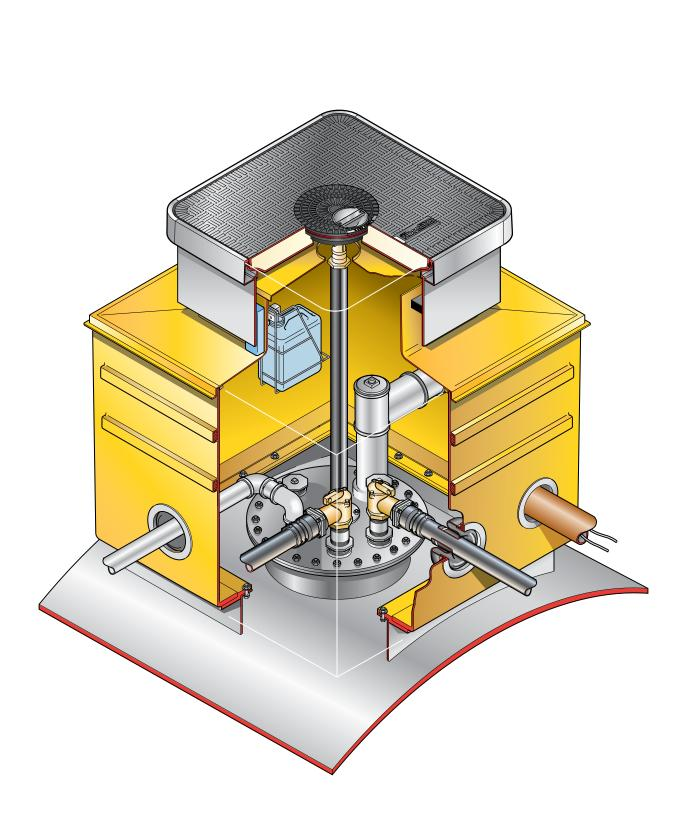
1.2m square bolted base chamber with a corbel, internal lid, adjustable skirt and square 760mm flat sealed cover with a central dip cover. (1m square tank flange connection).
