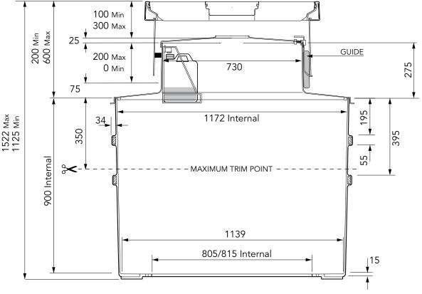
1.2m square bolted base chamber with a corbel, internal lid, adjustable skirt and square 760mm flat sealed cover with a central dip cover. (1m square tank flange connection).
