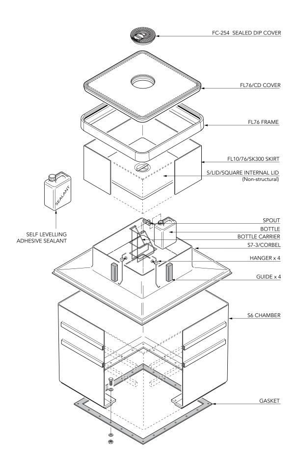
1.2m square bolted base chamber with a corbel, internal lid, adjustable skirt and square 760mm flat sealed cover with a central dip cover. (1m square tank flange connection).
