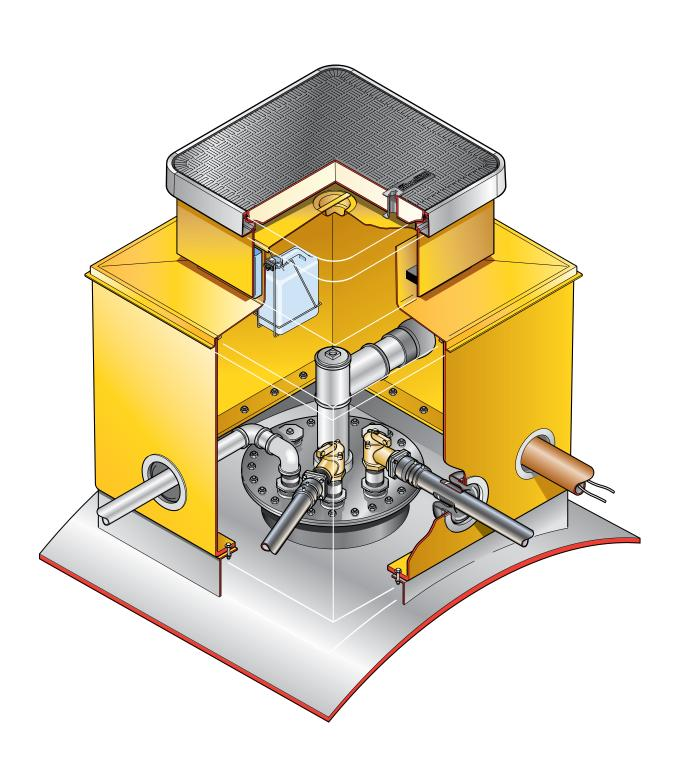
1.2m square base chamber with a sealed corbel, adjustable skirt and square flat sealed 760mm cover. 1.2m tank flange detail.
