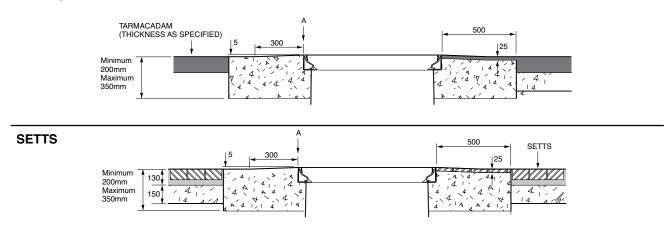
1.2m square base chamber with a sealed corbel, adjustable skirt and square flat sealed 760mm cover. 1.2m tank flange detail.
