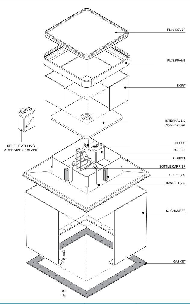
1.2m square base chamber with a sealed corbel, adjustable skirt and square flat sealed 760mm cover. 1.2m tank flange detail.
