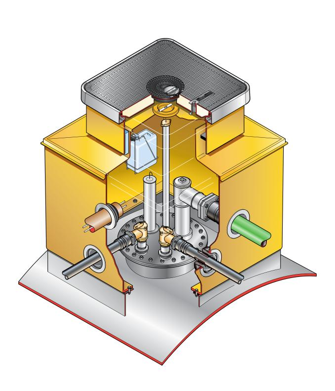
1.2m square base chamber with a sealed corbel, adjustable skirt, non-structural internal lid and square 760mm flat sealed cover with a central dip cover 1.2m square tank flange detail.
