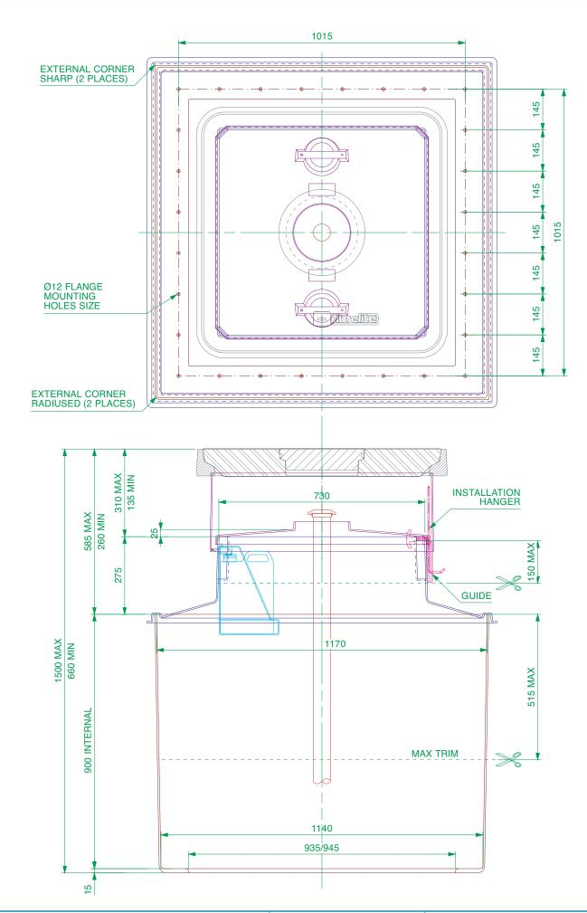
1.2m square base chamber with a sealed corbel, adjustable skirt, non-structural internal lid and square 760mm flat sealed cover with a central dip cover 1.2m square tank flange detail.
