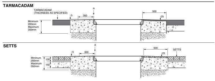
1.2m square base chamber with a sealed corbel, adjustable skirt, non-structural lid with central hole and round 900mm flat sealed cover with a central manual dip cover. (1.2m square tank flange detail)
