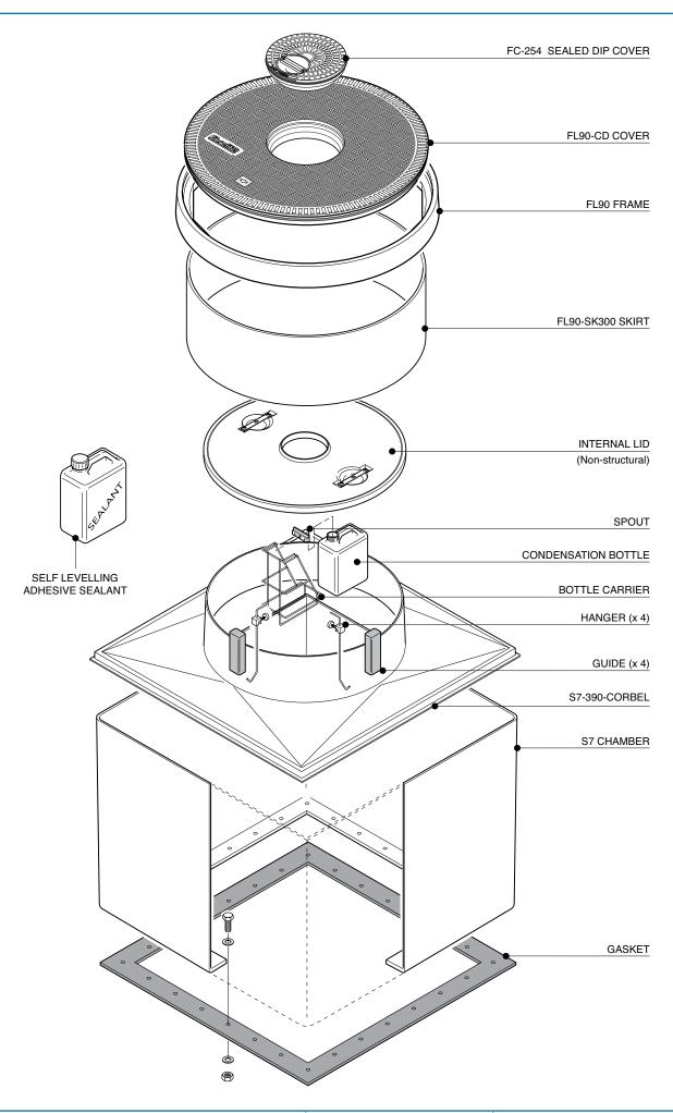
1.2m square base chamber with a sealed corbel, adjustable skirt, non-structural lid with central hole and round 900mm flat sealed cover with a central manual dip cover. (1.2m square tank flange detail)
