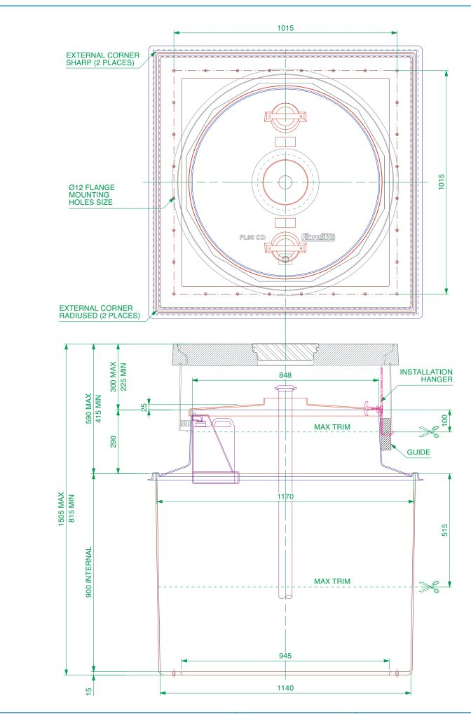
1.2m square base chamber with a sealed corbel, adjustable skirt, non-structural lid with central hole and round 900mm flat sealed cover with a central manual dip cover. (1.2m square tank flange detail)
