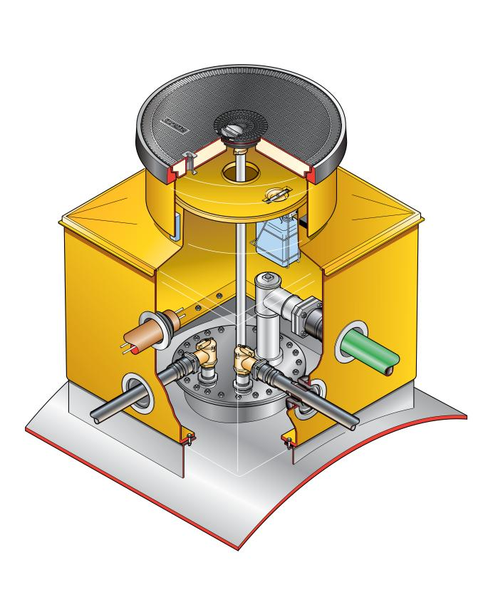
1.2m square base chamber with a sealed corbel, adjustable skirt, non-structural lid with central hole and round 900mm flat sealed cover with a central manual dip cover. (1.2m square tank flange detail)
