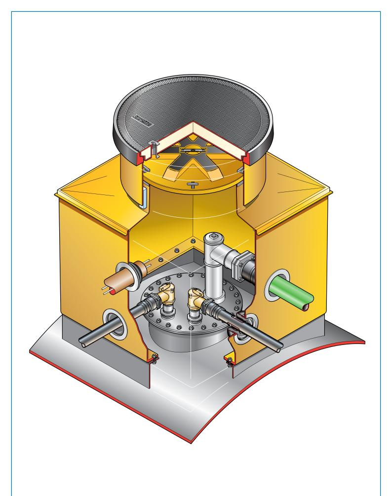
1.2m square base chamber with a sealed corbel, adjustable skirt, internal watertight platform and round 900mm flat sealed cover.  $1.2m^2$  tank flange detail
