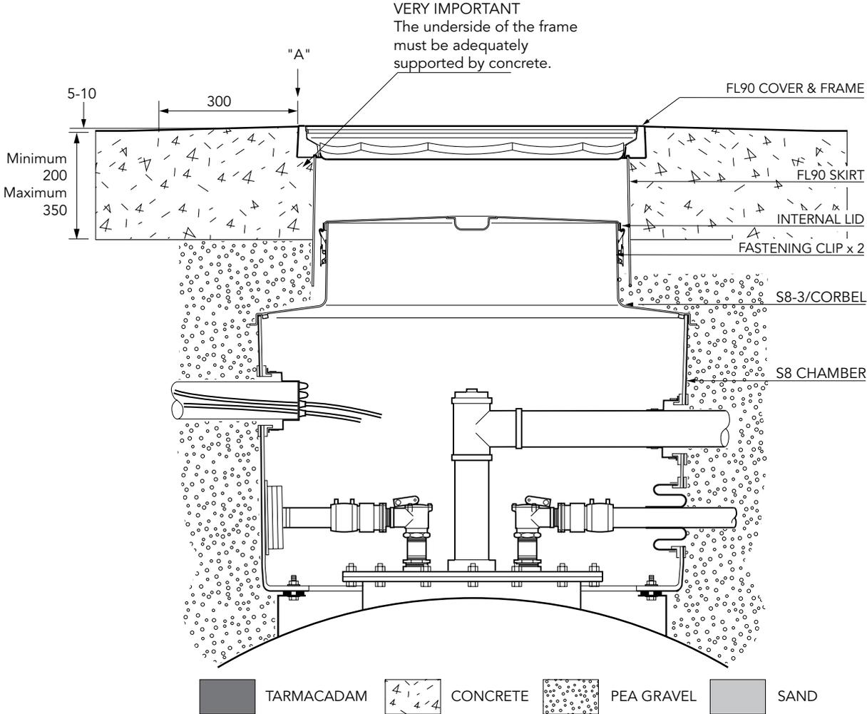
1.2m diameter bolted base chamber, corbel and internal lid with a watertight gasket and 2 fastening clips.
