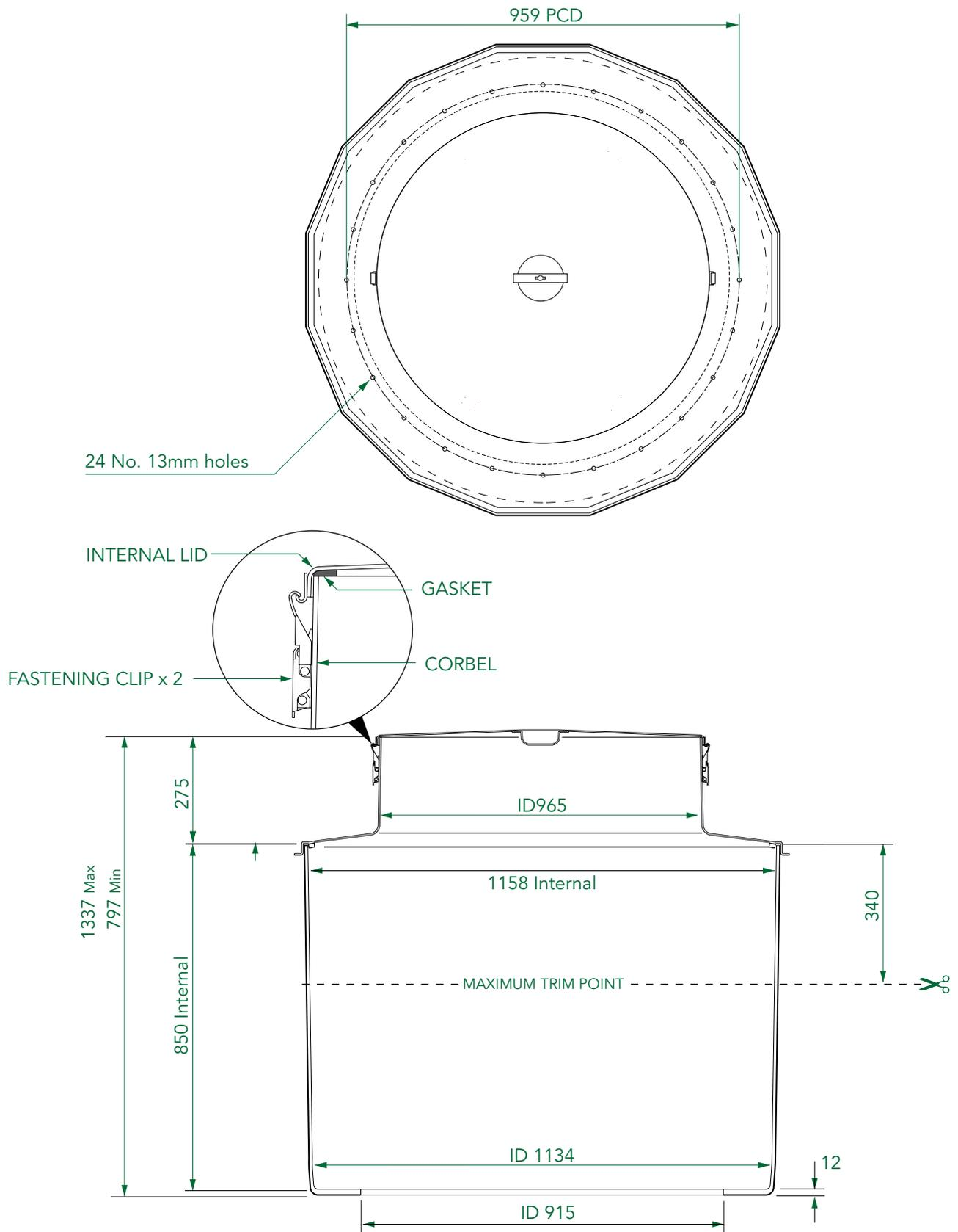
1.2m diameter bolted base chamber, corbel and internal lid with a watertight gasket and 2 fastening clips.
