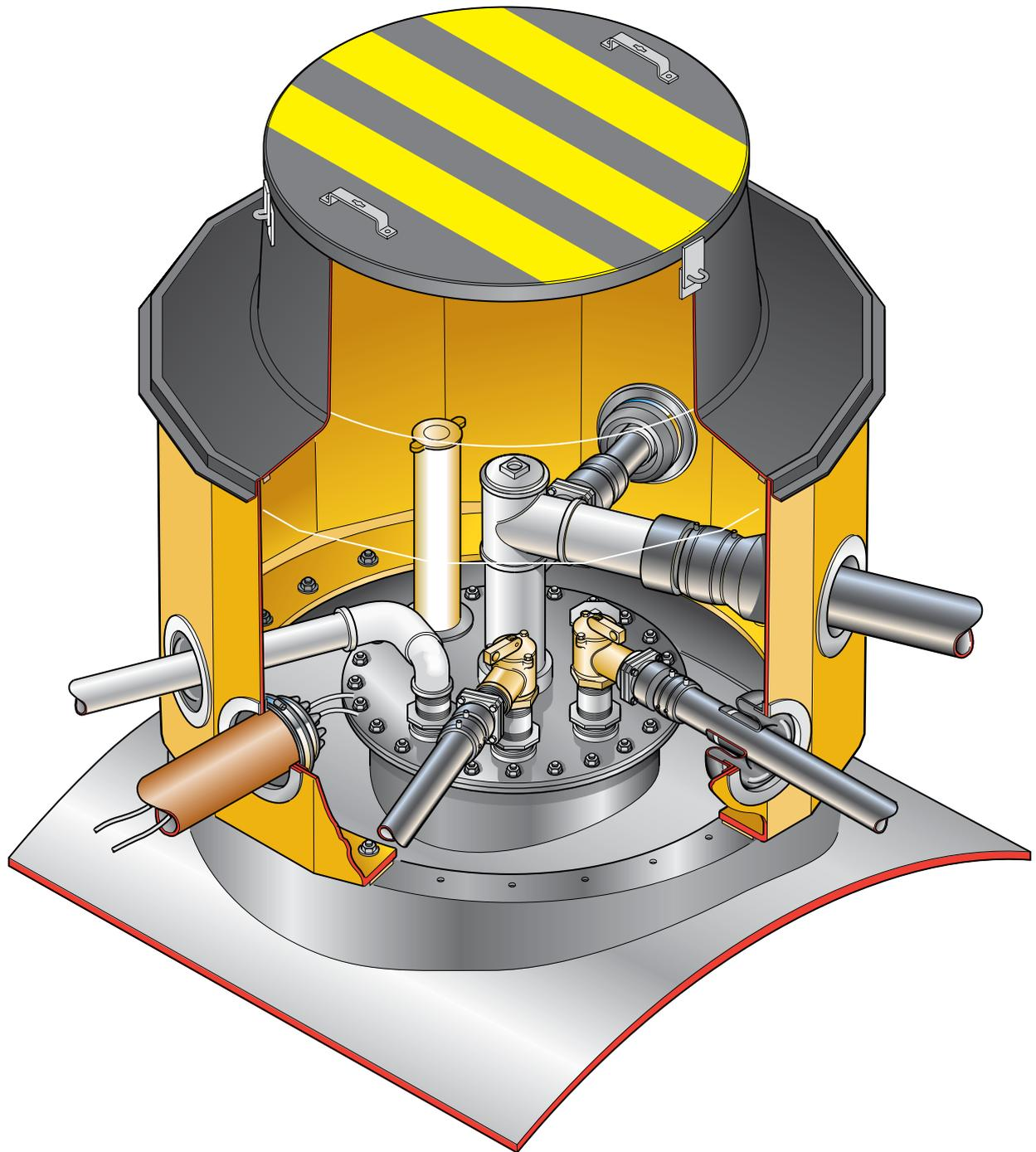
1.2m diameter bolted base chamber, corbel and internal lid with a watertight gasket and 2 fastening clips.
