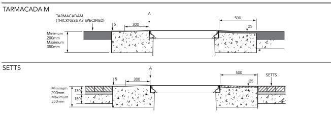
1.2m diameter chamber with a corbel, adjustable skirt and square 760mm flat sealed cover with central manul dip cover and frame. Round tank flange. Corbel/skirt sealkit.
