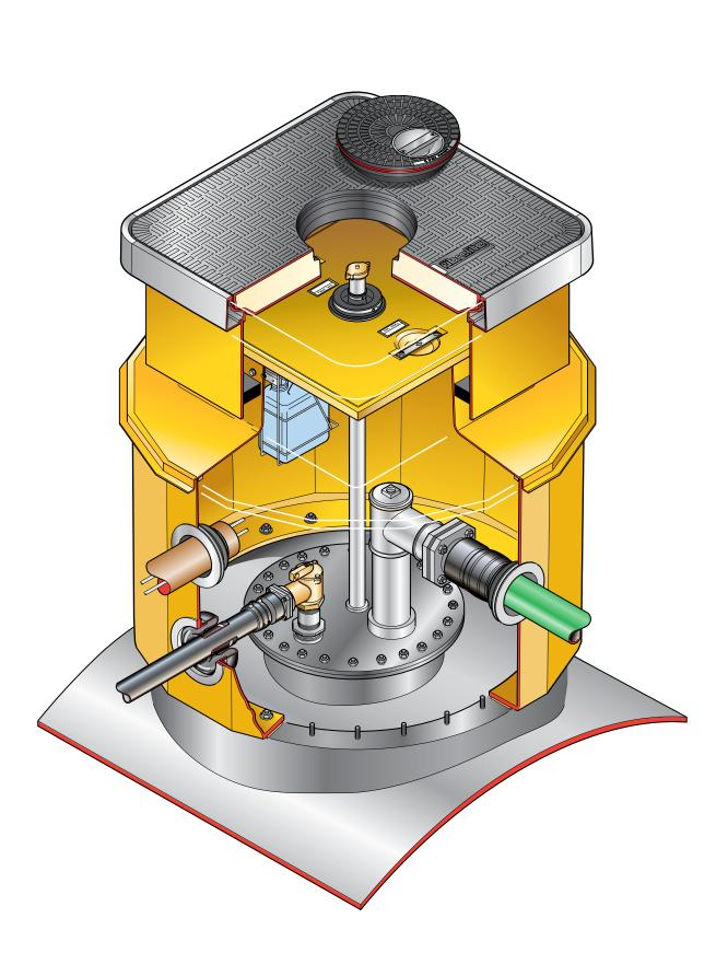
1.2m diameter chamber with a corbel, adjustable skirt and square 760mm flat sealed cover with central manul dip cover and frame. Round tank flange. Corbel/skirt sealkit.
