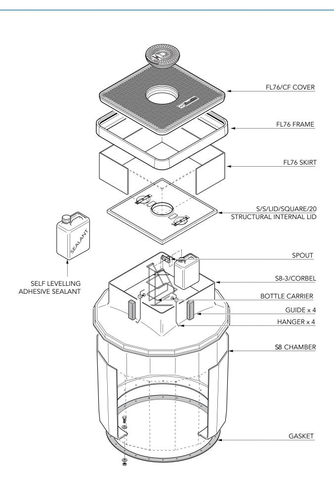
1.2m diameter chamber with a corbel, adjustable skirt and square 760mm flat sealed cover with central manul dip cover and frame. Round tank flange. Corbel/skirt sealkit.
