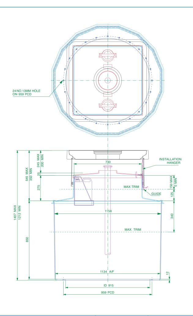
1.2m diameter chamber with a corbel, adjustable skirt and square 760mm flat sealed cover with central manul dip cover and frame. Round tank flange. Corbel/skirt sealkit.
