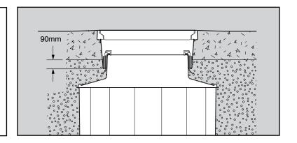
Complete backfilling to appropriate level. Frame must be supported by a minimum depth of 200mm of concrete Concrete ties must be inserted as close to the frame as possible. Minimum block of 500mm square around the frame. Joint must be tied as per diagram. Continuous pour preferred if possible.
