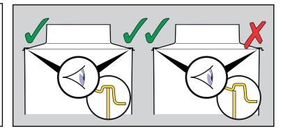
Measure distance between opposite walls, this should be 1158mm. If less than this you will need to brace out the sump.
