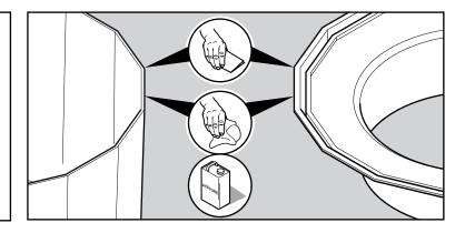
Dry fit the corbel on the sump to ensure it fits - push corbel groove onto sump wall.
