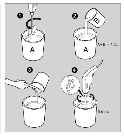
1 set of cans A+B will seal 2 sumps. Decant mixture from can A into can B to have more control when puring the mixture into the void, onto the sand base. Avoid spilling the contents to ensure a clean finish on the side walls of corbel and skirt. The sealant shall be poured to level 30mm below the top edge of the Corbel (the amount of sealant required is dependant on the height of the system but should be between 1.5
