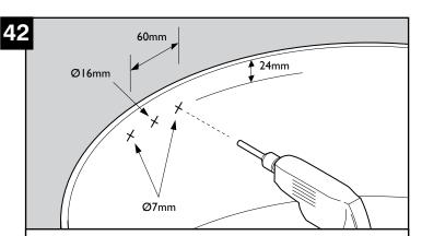
Mark out the position of the two holes to be drilled 24mm down from the top edge of the Corbel and 60mm cross centre. Drill the two Ø7mm holes into the Corbel walls.
