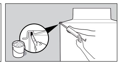
Seal around the outside joint and smooth off sealant with soapy water.
