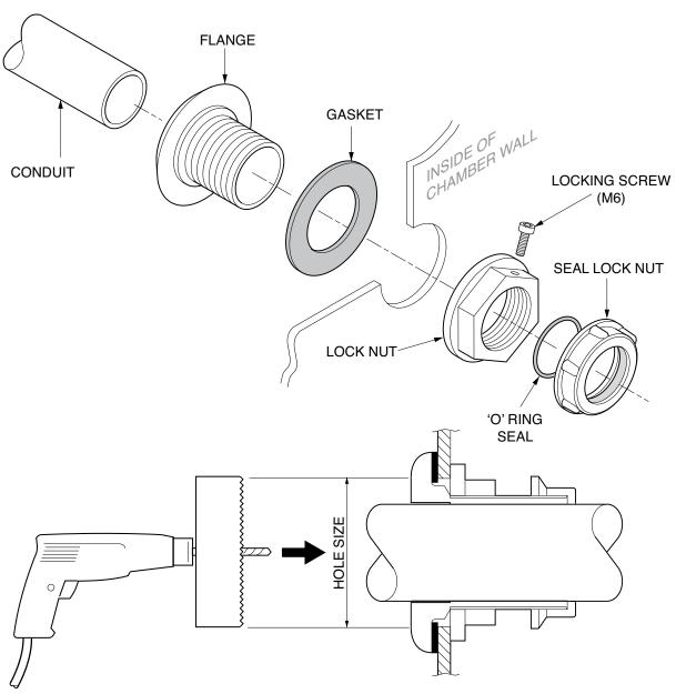
**NB:** Use the correct size drill piloted hole saw for each entry kit. The cable entry seal must be fitted perpendicular to the chamber wall and the conduit must enter the entry kit perfectly aligned. When backfilling ensure the conduit is not disturbed.
