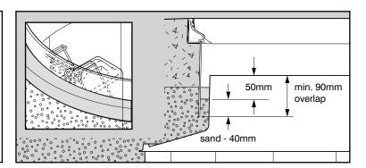
Drain and bottle should be positioned away from pipe risers and stp. The drain must be installed at the created low point to do this. Compact the sand in a way to create a low point 10-15mm lower than the surrounding sand.
