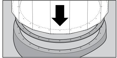
Fit a bolt and washer into each of the 24 holes (use only those supplied). Fit a washer and nut to each of the bolts. Tighten each bolt to 13.5Nm/10lbft torque, employing the following method, to avoid distortion of chamber.
