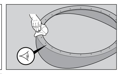
Remove protective cover from base of chamber and position chamber onto tank flange, aligning the holes. Ensure the seal on the base of chamber is not damaged and is free from grit etc.
