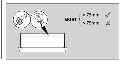
Ensure that you have a min overlap of 90mm between the skirt and corbel, to allow space to install the seal kit.
