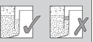
Ensure void is free of concrete to a depth of 90mm (120mm on a high water table installation).
