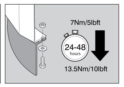
Starting with any bolt tighten to 7Nm/5lbfft torque. Move to the bolt positioned at 180° and tighten to 7Nm/5lbffttorque. Move 180° plus one bolt pitch and tighten to 7Nm/5lbfft of torque. Repeat until all bolts are tightened to 7Nm/5lbfft torque. Now repeat the procedure tightening all bolts to 13.5Nm/10lbfft torque.
