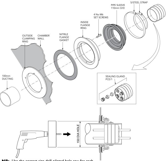
**NB:** Use the correct size drill piloted hole saw for each entry kit. The cable entry seal must be fitted perpendicular to the chamber wall and the conduit must enter the entry kit perfectly aligned. When backfilling ensure the conduit is not disturbed.
