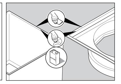
Dry fit the corbel on the chamber to ensure it fits - push corbel groove onto chamber wall,
