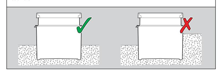
Complete backfilling to appropriate level. Frame must be supported by a minimum depth of 200mm of concrete.
