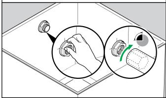
7 Tighten the locking screw with a 5mm Allen key
