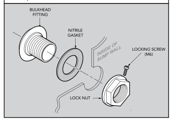
Initially hand tighten the lock nut until it is hand tight (ensure that the locking screw is accessible post installation), then using the supplied box spanner tighten the lock nut an additional 1/4 - 1/2 a turn. DO NOT OVER TIGHTEN AS THIS MAY DAMAGE THE FITTING.
