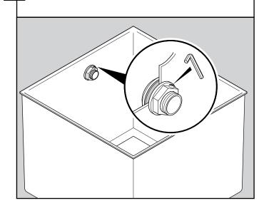
Push the conduit through the electrical cable entry seal and seal the conduit with the 'O' ring and seal nut.
