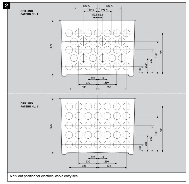
The electrical cable entry seal should be positioned perpendicular to the sump wall and the conduit must enter the electrical cable entry seal as aligned as possible.
