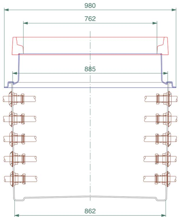
862mm x 862mm x 675mm deep solid base sump with a corbel and 760mm dia. flat sealed cover and frame.
