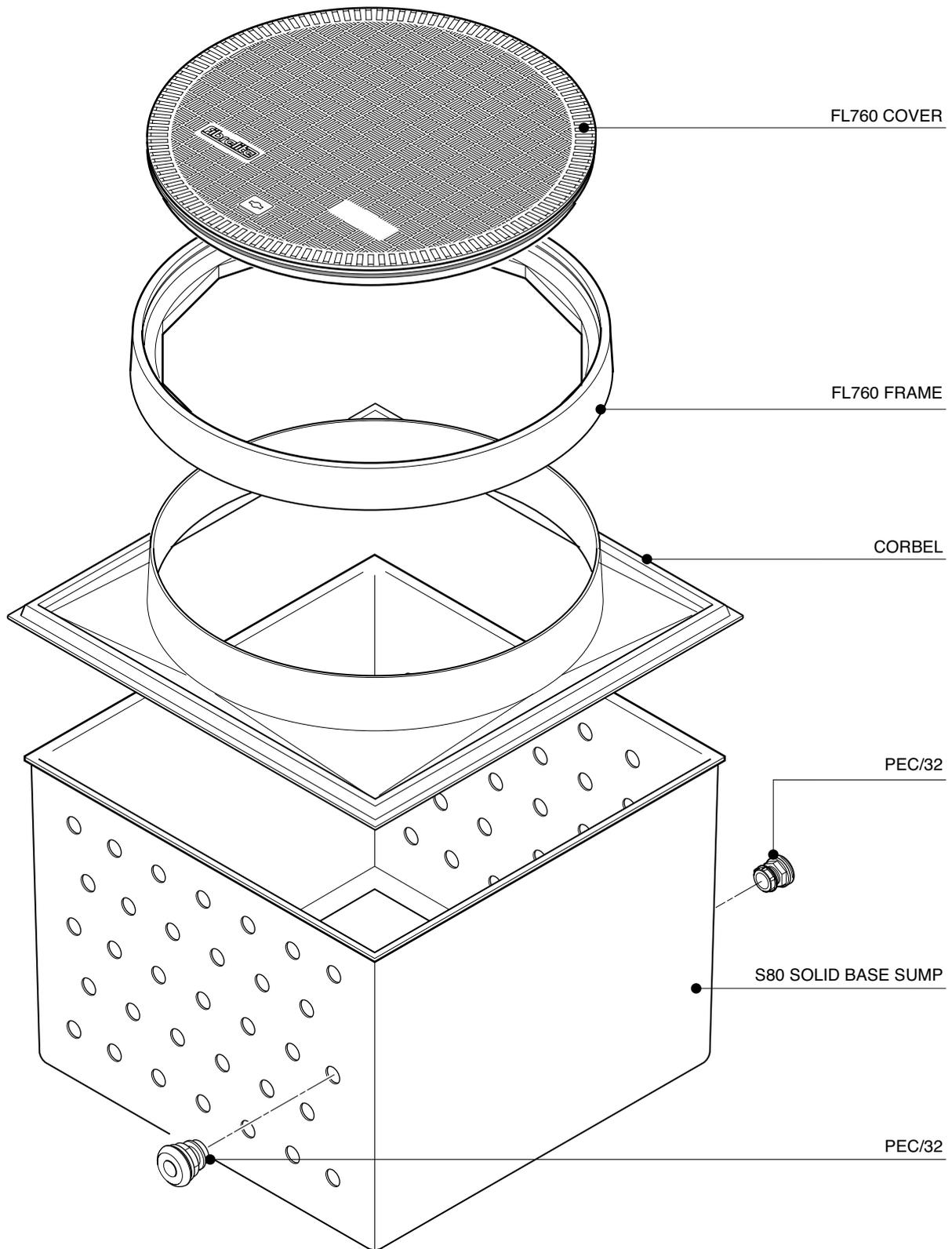
862mm x 862mm x 675mm deep solid base sump with a corbel and 760mm dia. flat sealed cover and frame.
