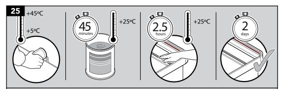
Application Temperature : +5 to +45 degrees °C (DO NOT apply at temperatures below +4 degrees °C)
