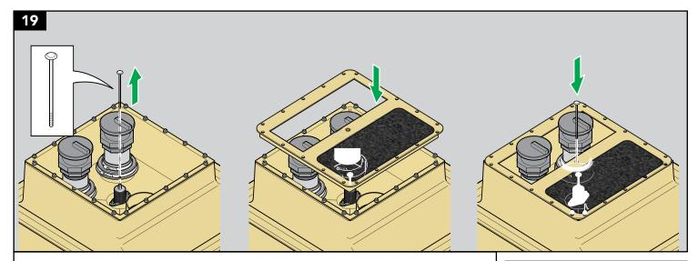
Seat the platform onto the spill container. If the system includes a drainback with an extended drainback plunger, remove the plunger and then refit the plunger.
