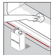
Degrease the outside surface of the corbel and the inside surface of the skirt with a suitable degreasing agent such as Acetone.
