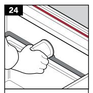
Decant a suitable amount of mixed sealant into a smaller tin/pot (DO NOT USE THE TIN THAT CONTAINED PACK "B") and pour the mixed sealant into the void between the corbel turret & skirt.
