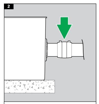
Connect the outside pipework to the pipe stubs using a welding socket and weld pipes.
