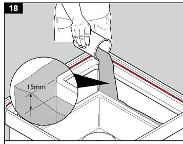
Sprinkle sand into the space between the outside of the corbel and the inside surface of the skirt. The distance from the top of the sand to the top of corbel should be 15mm.
