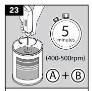
Mix contents together for a full 5 minutes using a slow speed electric drill (400-500rpm) with a low viscosity mixing paddle until a completely homogeneous mix is obtained. Mixing is made easier if pack (B) is added in two stages.
