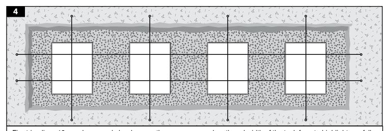
Fix string lines 10mm above grade level across the sump - across length and width of the tank farm to highlight any falls.
