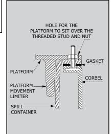
**NB:-** The platform is NOT bolted down to the spill container/sump but is sat over the threaded studs and nuts.
