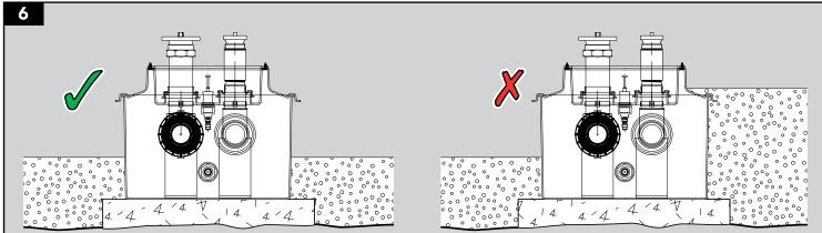
Once the corbel test has been performed with a PASS result, the area around the sump can be carefully backfilled with peagravel or sand. Back-fill equally around the sump in layers to prevent damage or deformation.
