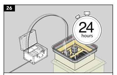
Wait 24 hours after the sealant has been poured between the sump and skirt, before performing a vacuum test.
