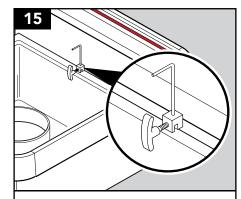
Set frame to the correct height using the hanging rods.
