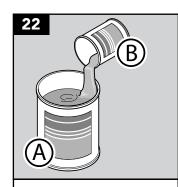
Stir the **COMPLETE** contents of pack (B) into the tin containing pack (A) to give a combined content of 4.5 litres.
