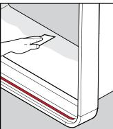
Thoroughly abrade the outside surface of the corbel and the inside surface of the skirt.
