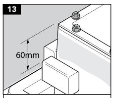
Fix the foam spacer blocks to the outside of the corbel at the height of 60mm.
