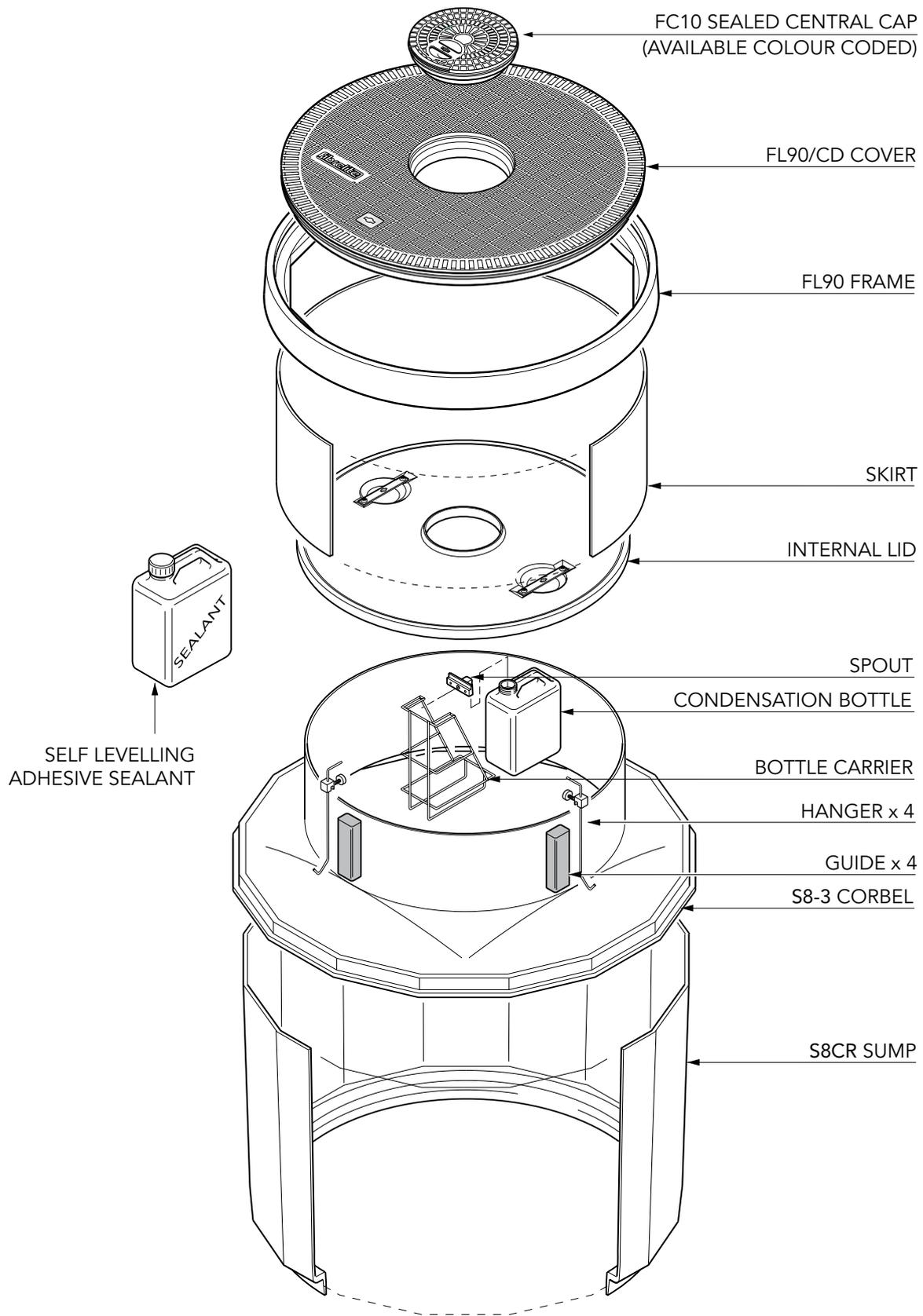
1.2m diameter chamber with collar ring base connection, a sealed corbel, internal lid, adjustable skirt and round 900mm flat sealed cover with a removeable central cap (254mm diameter) and composite frame.
