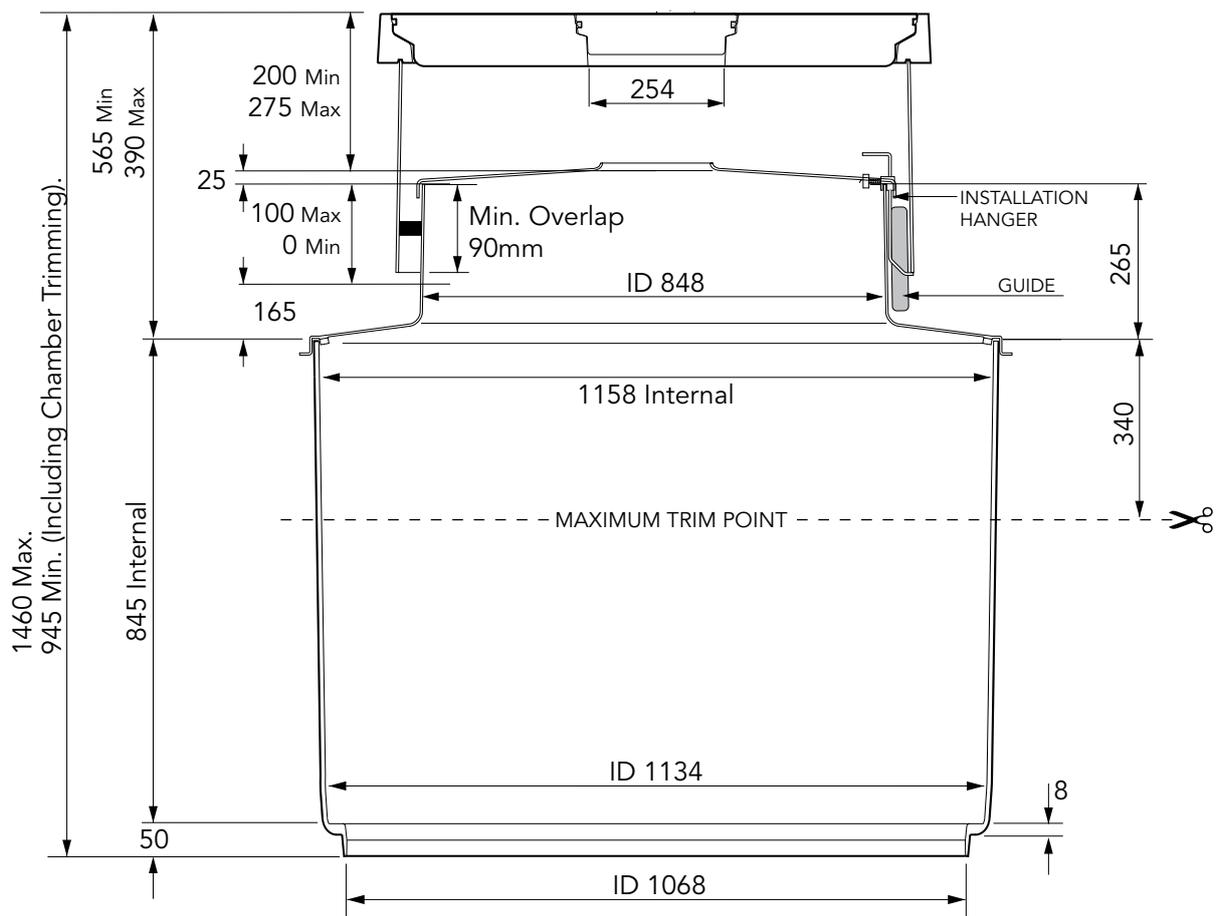
1.2m diameter chamber with collar ring base connection, a sealed corbel, internal lid, adjustable skirt and round 900mm flat sealed cover with a removeable central cap (254mm diameter) and composite frame.
