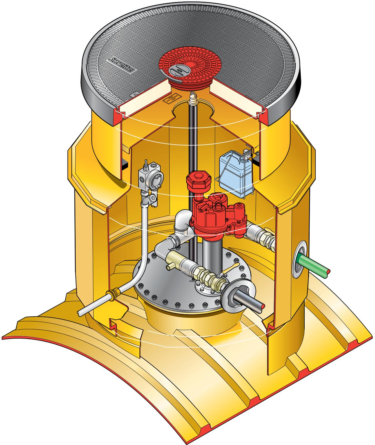
1.2m diameter chamber with collar ring base connection, a sealed corbel, internal lid, adjustable skirt and round 900mm flat sealed cover with a removeable central cap (254mm diameter) and composite frame.
