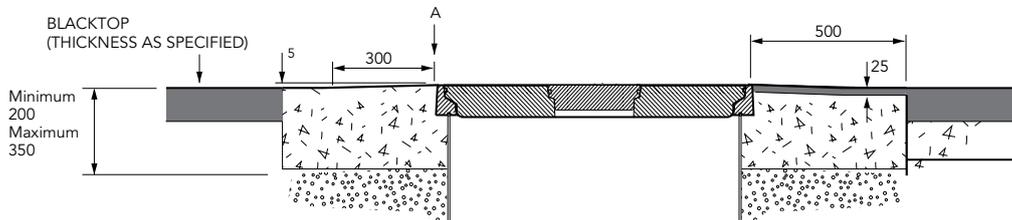
1.2m diameter chamber with collar ring base connection, a sealed corbel, internal lid, adjustable skirt and round 900mm flat sealed cover with a removeable central cap (254mm diameter) and composite frame.
