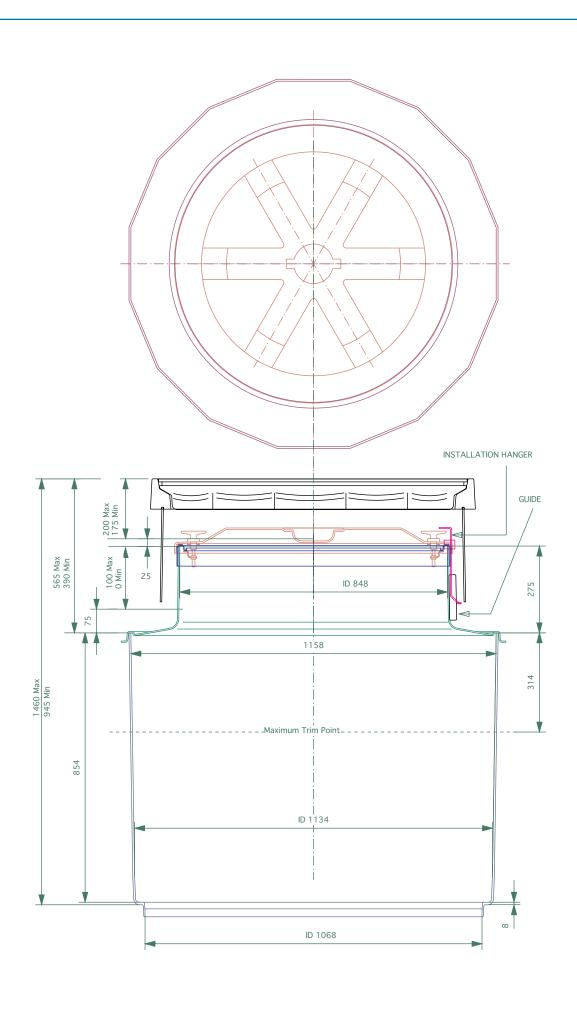
1.2m diameter chamber with collar ring base connection, a sealed corbel, watertight platform, adjustable skirt and round 900mm flat sealed cover and composite frame.
