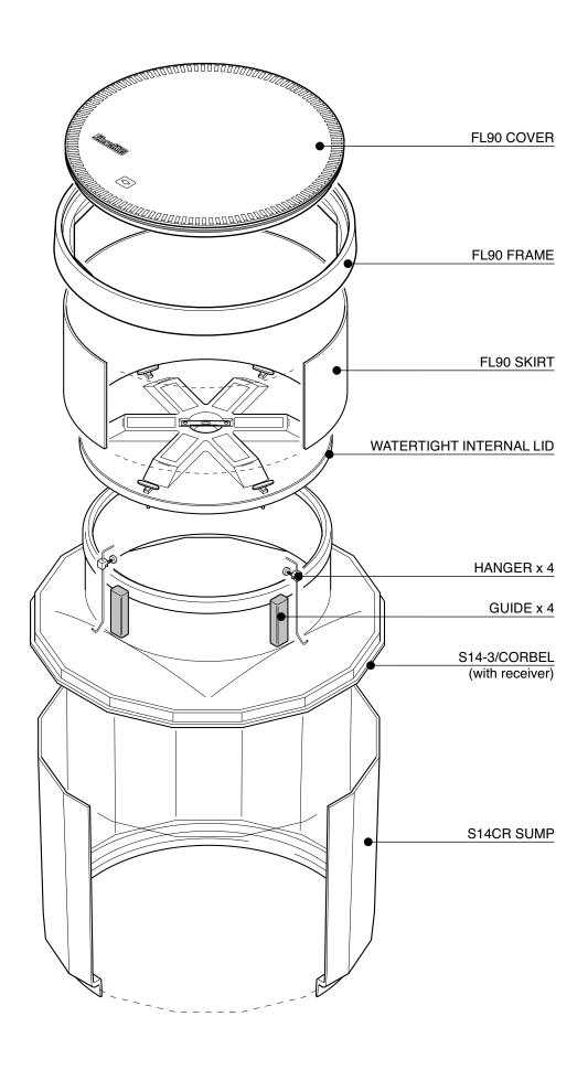
1.2m diameter chamber with collar ring base connection, a sealed corbel, watertight platform, adjustable skirt and round 900mm flat sealed cover and composite frame.
