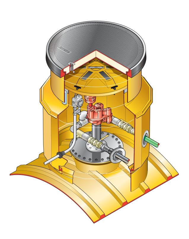
1.2m diameter chamber with collar ring base connection, a sealed corbel, watertight platform, adjustable skirt and round 900mm flat sealed cover and composite frame.
